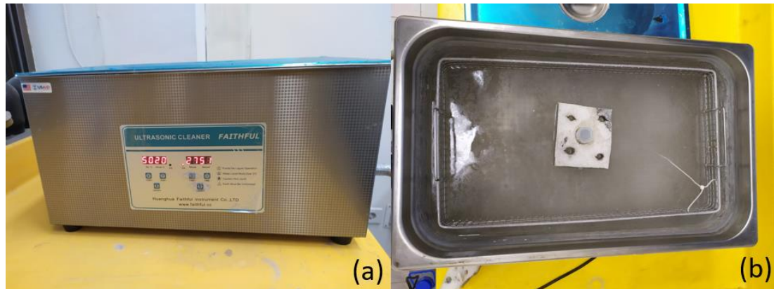
Figure 4-2 Sonicator (a) front view (b) top view
