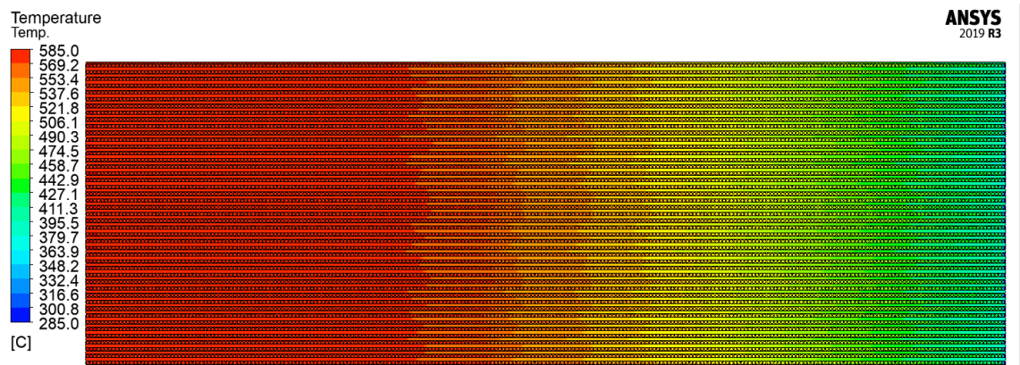
Figure 4-3 Temperature contours of TESS at t=60 min, Case-I, Charging
