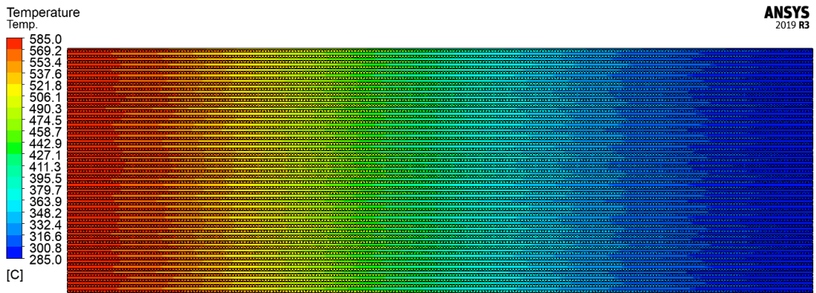
Figure 4- 1 Temperature contours of TESS at t=30 min, Case-I, Charging
