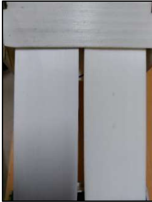
Figure 34: Resin 3d printed Flap Surface (Prototype V2)
