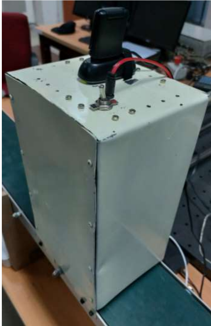
Figure 27: Sheet metal enclosure for lighting and camera deployment (Image)
