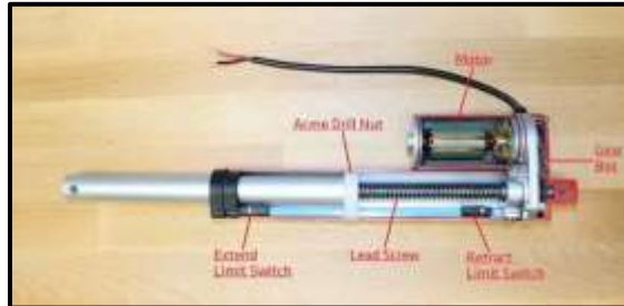
Figure 4: DC Motor operated Linear Actuator [15]
