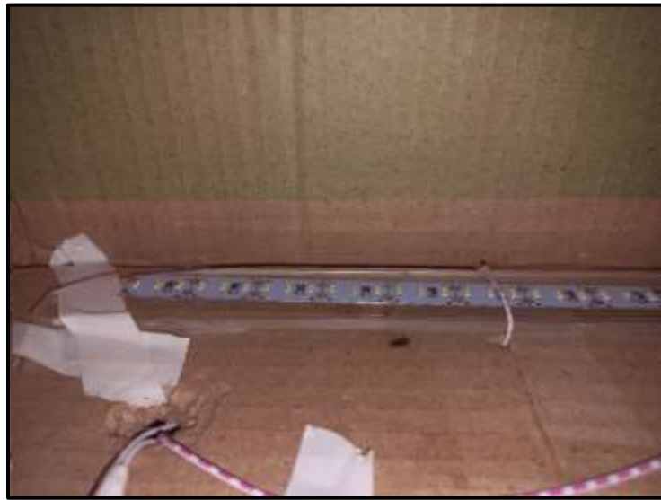
Figure 25: Heat sink for LED strip lights
