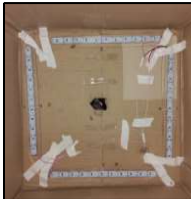
Figure 24: LED Strip Lights installed on roof of cardboard enclosure
