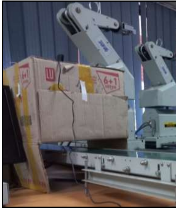
Figure 23: Cardboard Enclosure installed on Lab Conveyor Belt
