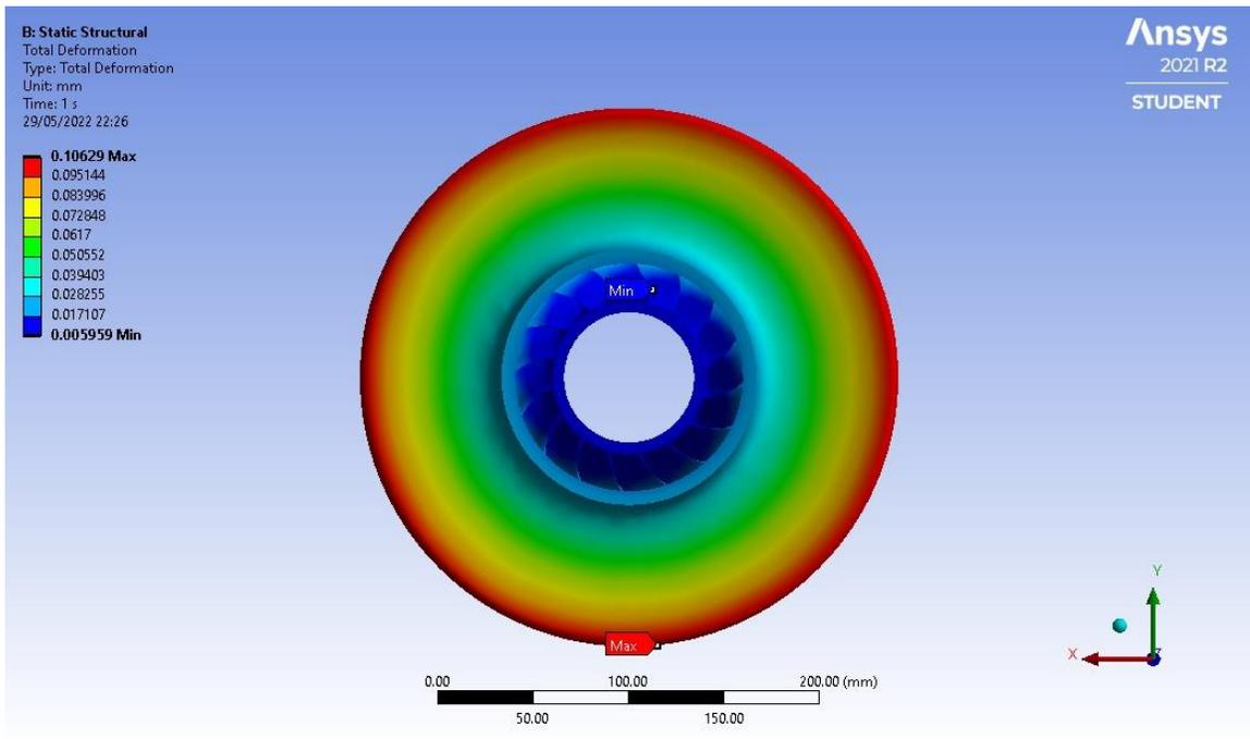
**Figure 23: Total Deformation of Impeller**
