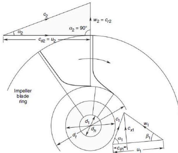
**Figure 6: Velocity Diagram for radial blades**
