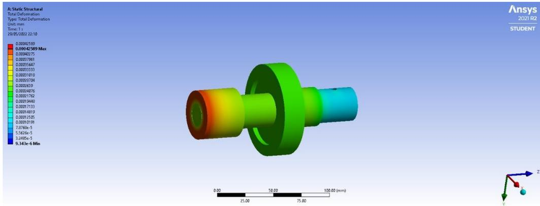
**Figure 29: Total Deformation**
