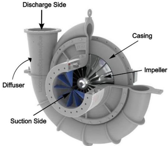
The centrifugal compressor is one of the most popular types of air compressors. It uses a rotating impeller or disc in the casing to push the gas or air towards the impeller blades. The impeller blades increase the speed of the gas. The diffuser converts the gas velocity energy into pressure. After that, the gas is directed to the desired location.
