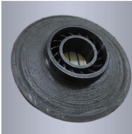
**Figure 33: Physical Impeller**
