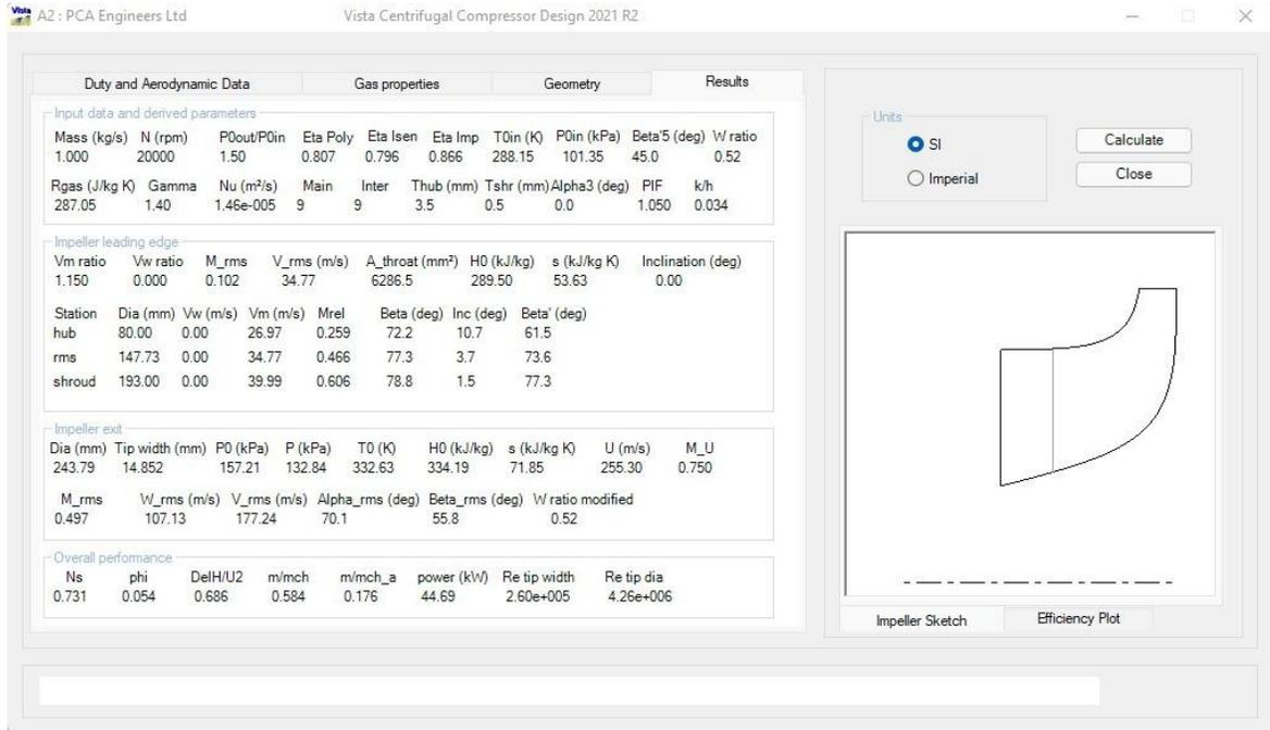
*Figure 11: Input Data and Derived Parameters*
