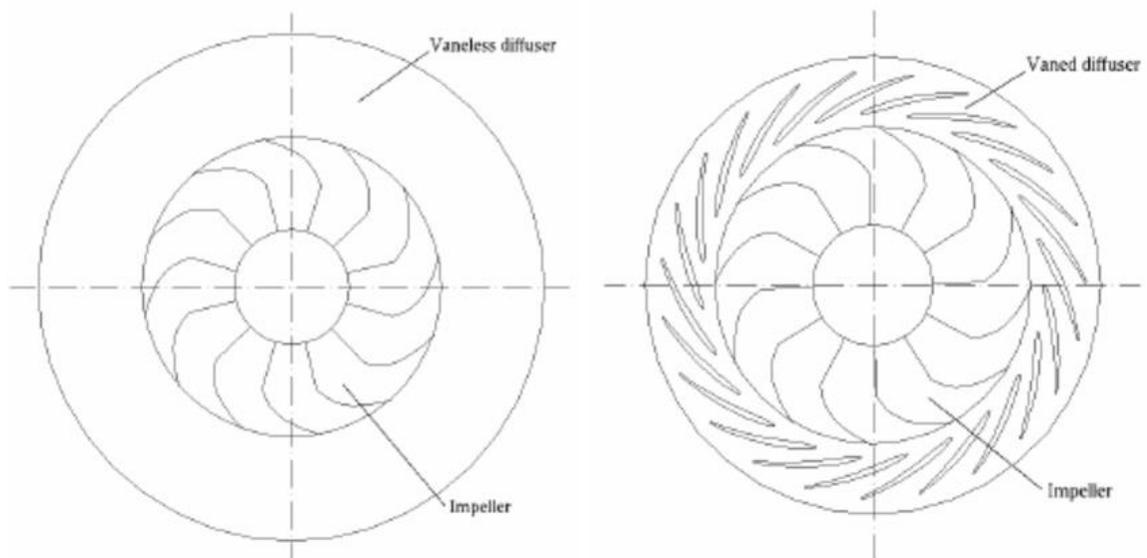
**Figure 2: Vanless and Vaned Diffuser**
