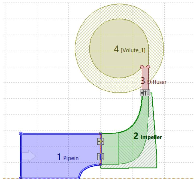
**Figure 9: Meridional Figure of compressor from CFTurbo**
