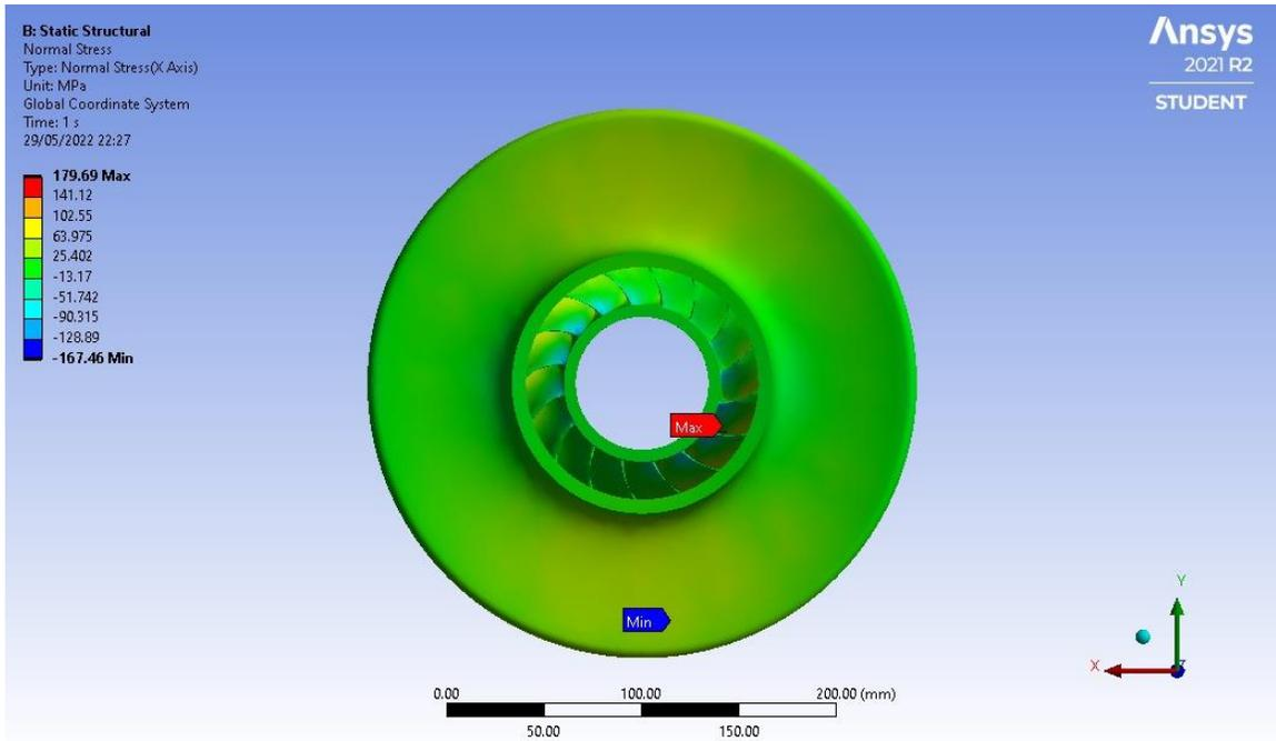
**Figure 26: Normal Stress in X-axis**
