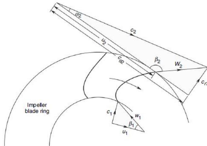
**Figure 8: Velocity Diagram for Backward blade impeller**
