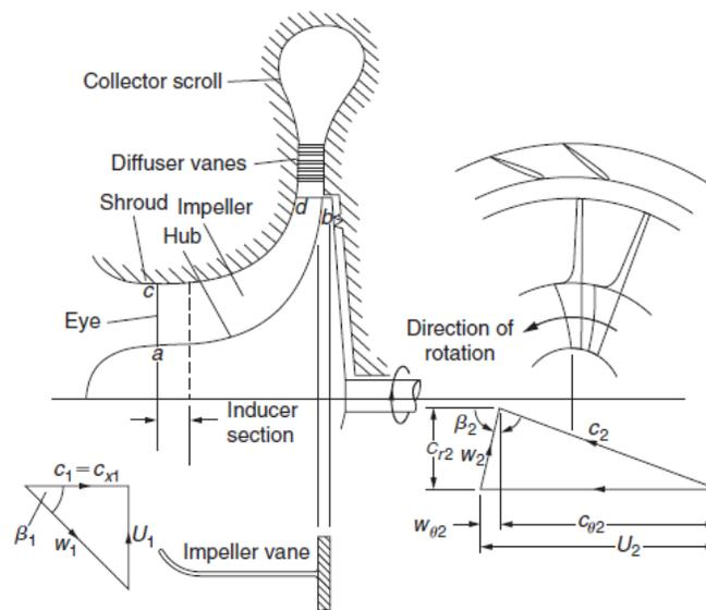
**Figure 4: Impeller of compressor**
