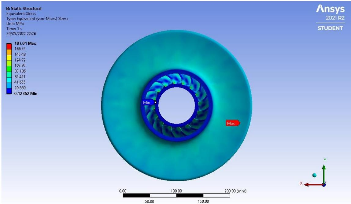
**Figure 24: Equivalent Stress on Impeller**
