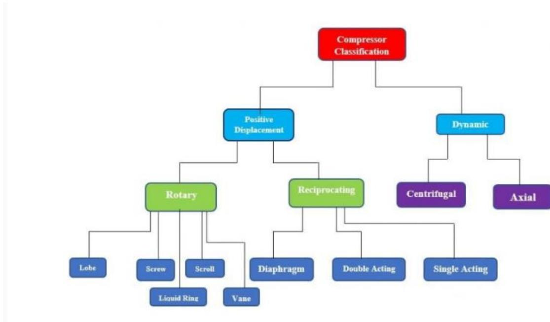
**Figure 1: Types of Compressors**
