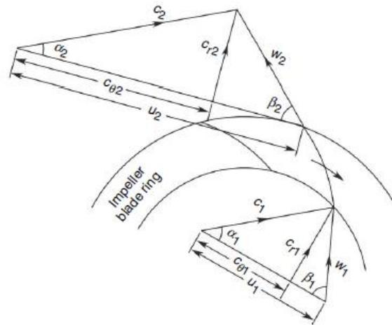
**Figure 7: Velocity Diagrams for forward blade impeller**
