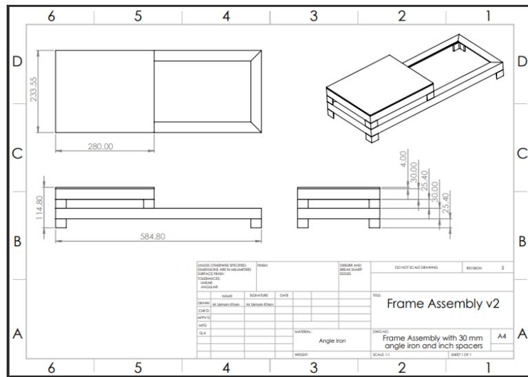
**Figure 42: Drawing for frame of Assembly**
