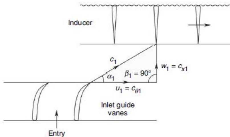
**Figure 5: Inlet Guide Vanes usage**
