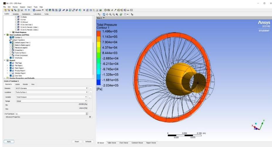
**Figure 21: Pressure Distribution on Blade Profile**
