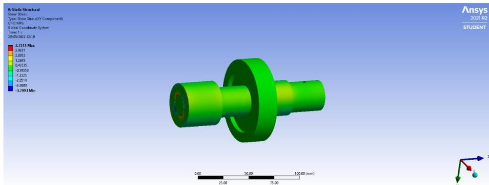
**Figure 31: Shear Stress on Shaft**
