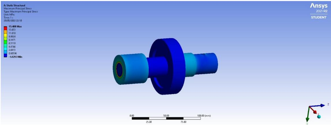
**Figure 32: Maximum Principal Stress on Shaft**
