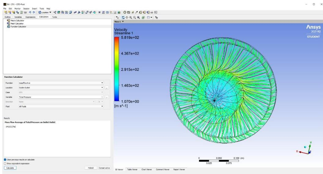
**Figure 22: Velocity Distribution on Blade Profile**
