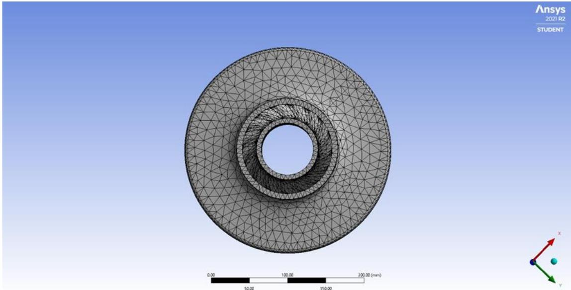
**Figure 18: Meshed Body of Impeller**
