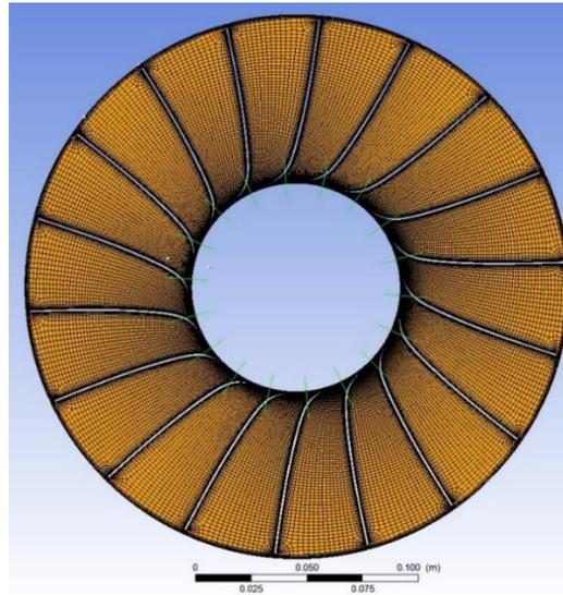
**Figure 16: Meshed Impeller for CFD**
