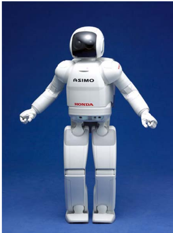
Figure 4 ASIMO - A fully actuated humanoid robot by Honda
