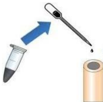
Figure 0.3 Coating of slurry on GCE
