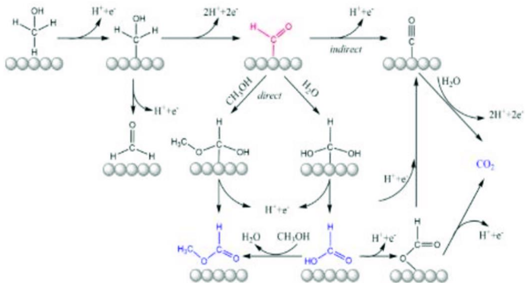
Figure 0.6 Proposed mechanism of methanol oxidation reaction
