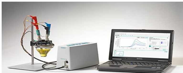
Figure 0.2 Illustrated diagram of electrochemical workstation
