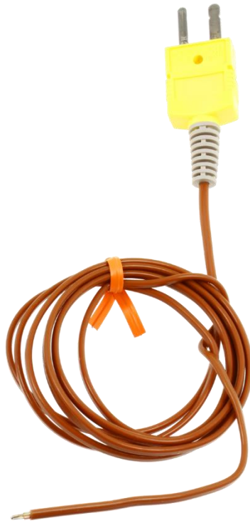
Figure 3.2 K-Type thermocouple for temperature measurements.
