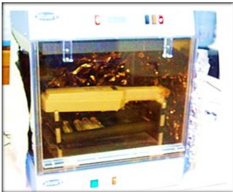
Fig. 3.6: Photocatalysis at 40 °C Temperature with Pure TNPs
