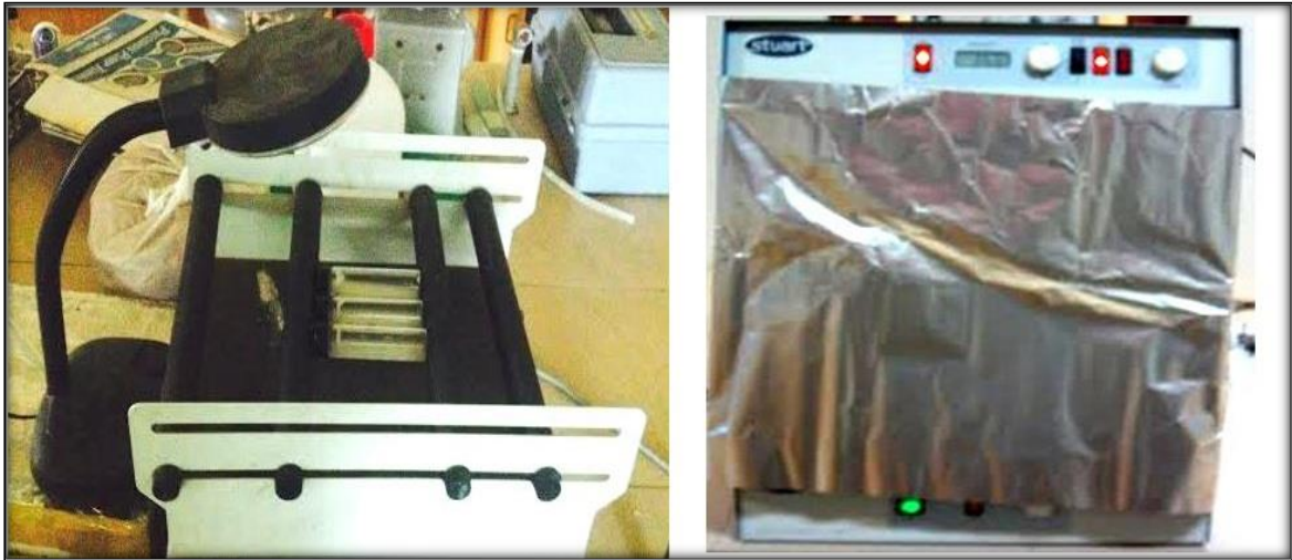
Fig. 3.7: Photocatalysis with silver doped TNPs at Room Temperature and 40 °C
