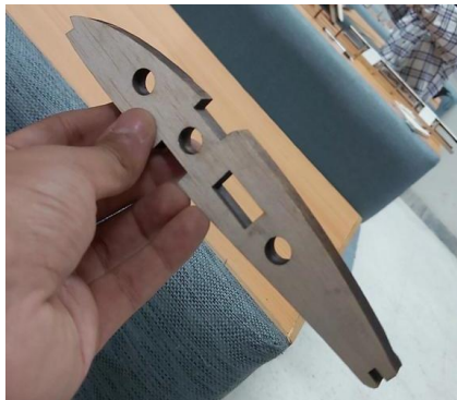
Figure 32: Finished Laser Cut Rib
