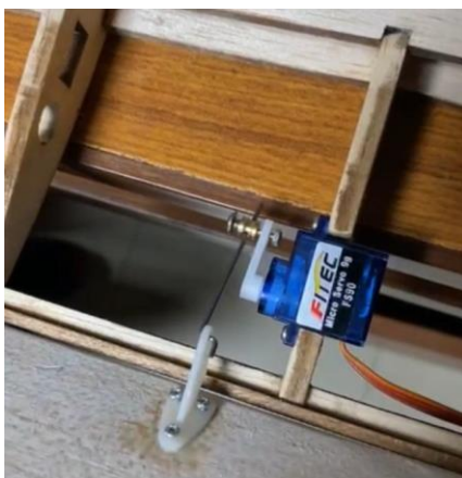
Figure 39: The lever-push rod-crown-horn apparatus
