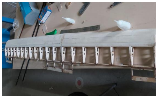
Figure 35: Completed Wing Assembly
