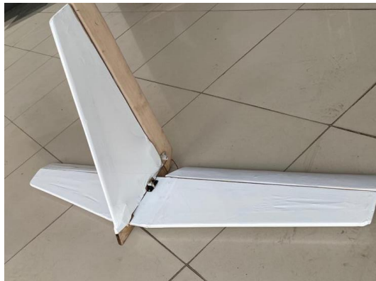
Figure 42: Solar Foil sheeted tail
