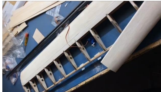
Figure 38: Flaps with Hinges on Wing
