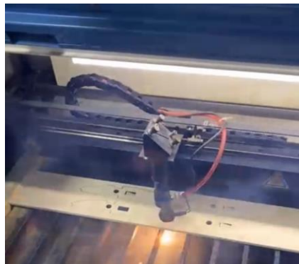
Figure 31: Laser Cutting of 10mm Plank for Wing Rib
