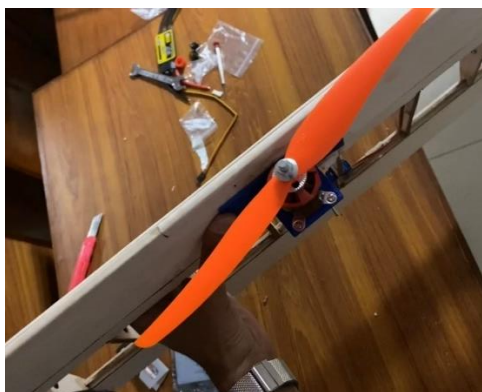
Figure 40: BLDC Mount with Propeller
