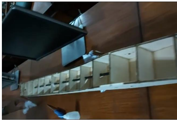
Figure 37: Carbon Fiber Rod in Fuselage
