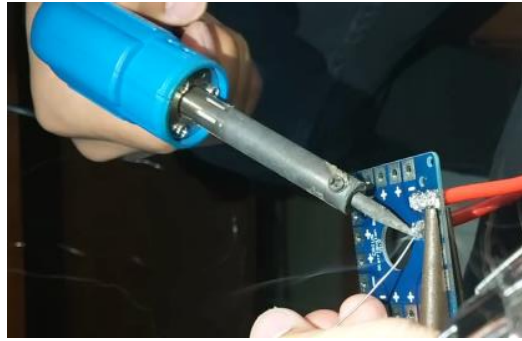
Figure 49: Power Distribution Board being soldered
