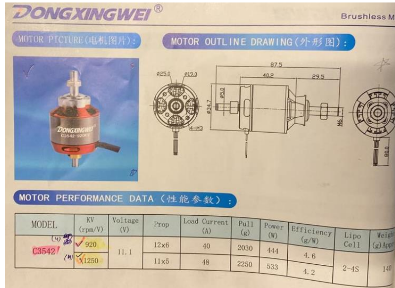
Figure 66: BLDC Specifications and drawing
