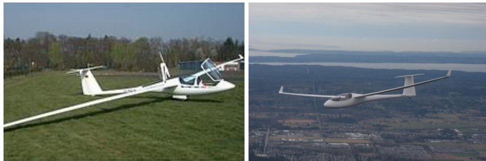
Figure 8: ASH 25 (left) with AR = 39.8 & HP-24 (right) with AR = 23.
