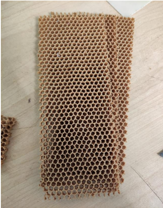
Figure 7: Honeycomb (5mm thick)
