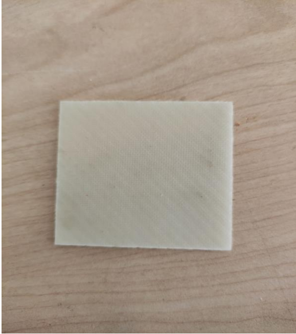
Figure 6: 6-layered Glass Fiber Face sheet
