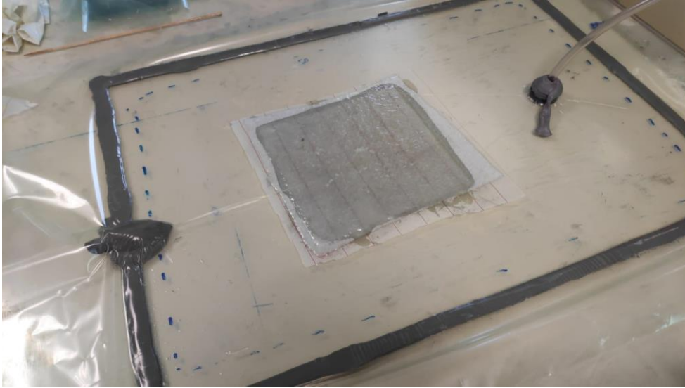
Figure 2: Adhesive getting dry under vacuum
