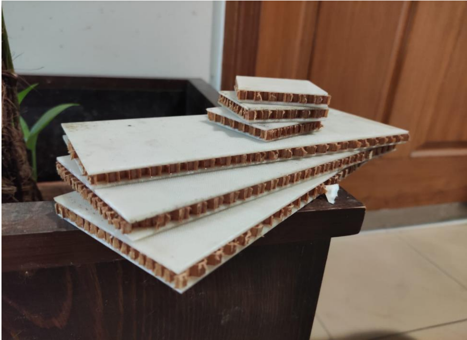
Figure 9: Sandwich structures without any Nano-Particles
