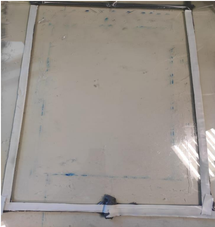
Figure 5: PVA applied to the working area
