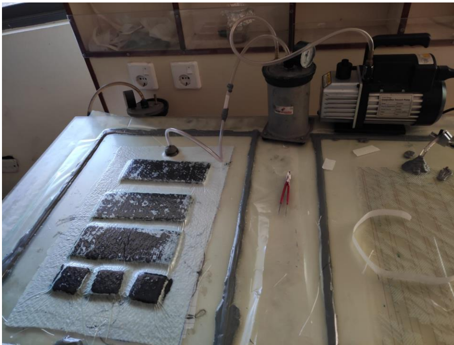
Figure : Adesive with CNTs getting dry under vacuum
