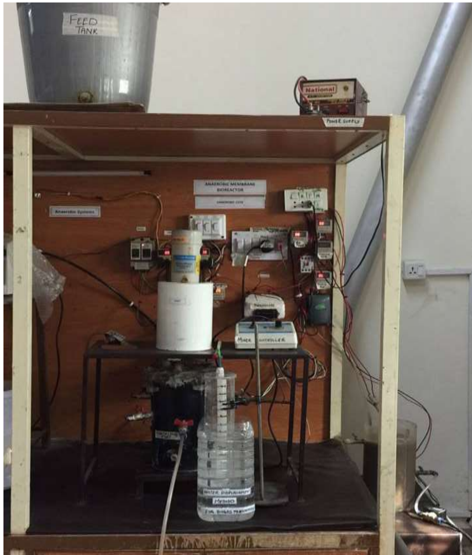
Figure 3.1 Anaerobic- Aerobic SBR system
