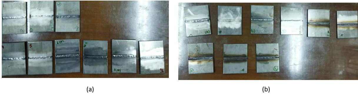
Figure 3-3: Specimens welding (a) AISI321/ER316L Filler (b) AISI321/ER308L Filler
