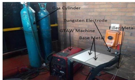
Figure 3-2: TIG Welding Setup
