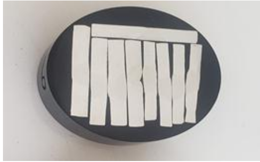
Figure 3-7: Mounted Sample (ER316L)
