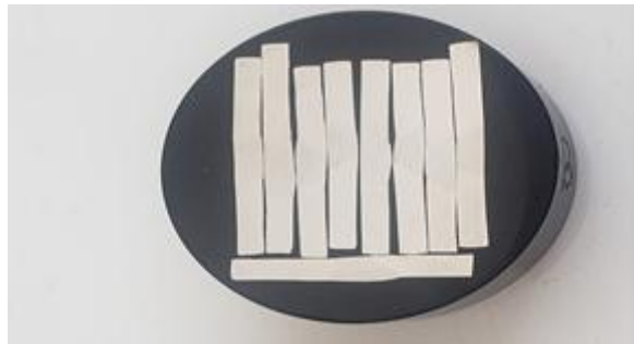
Figure 3-7: Mounted Sample (ER316L)
