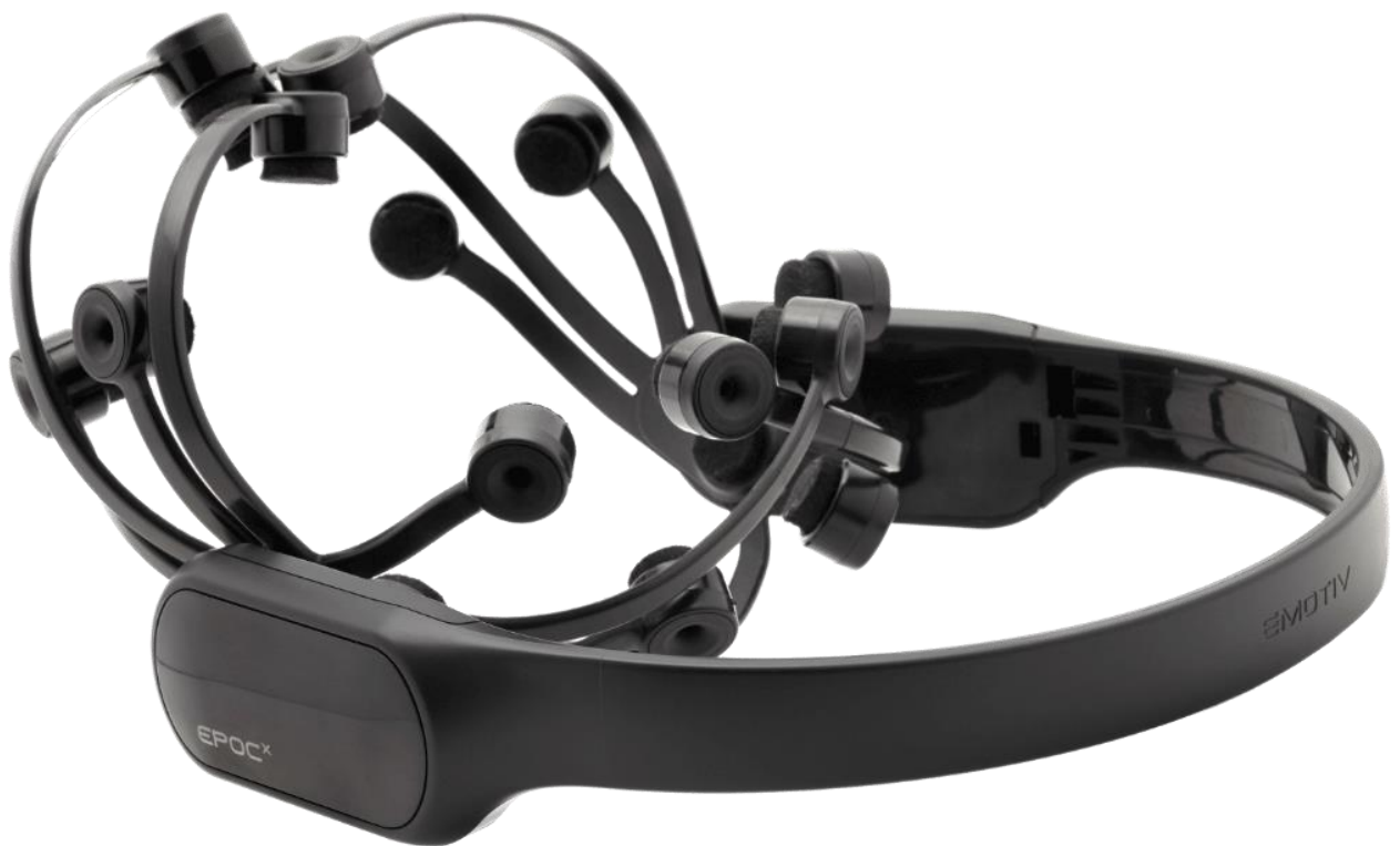
Figure 1: A 14-channel EMOTIV EEG headset
