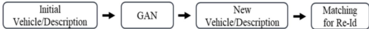
Figure 3: Vehicle re-identification system based on GAN: This image shows the visual layer of GAN usage for Vehicle re-identification , Visual description of vehicle is learned by Generator after frequent matching with discriminator and then new learned description is used for matching of vehicle for vehicle re-id [29].
