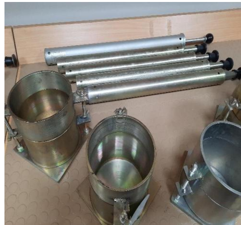
d) Proctor Test Apparatus
