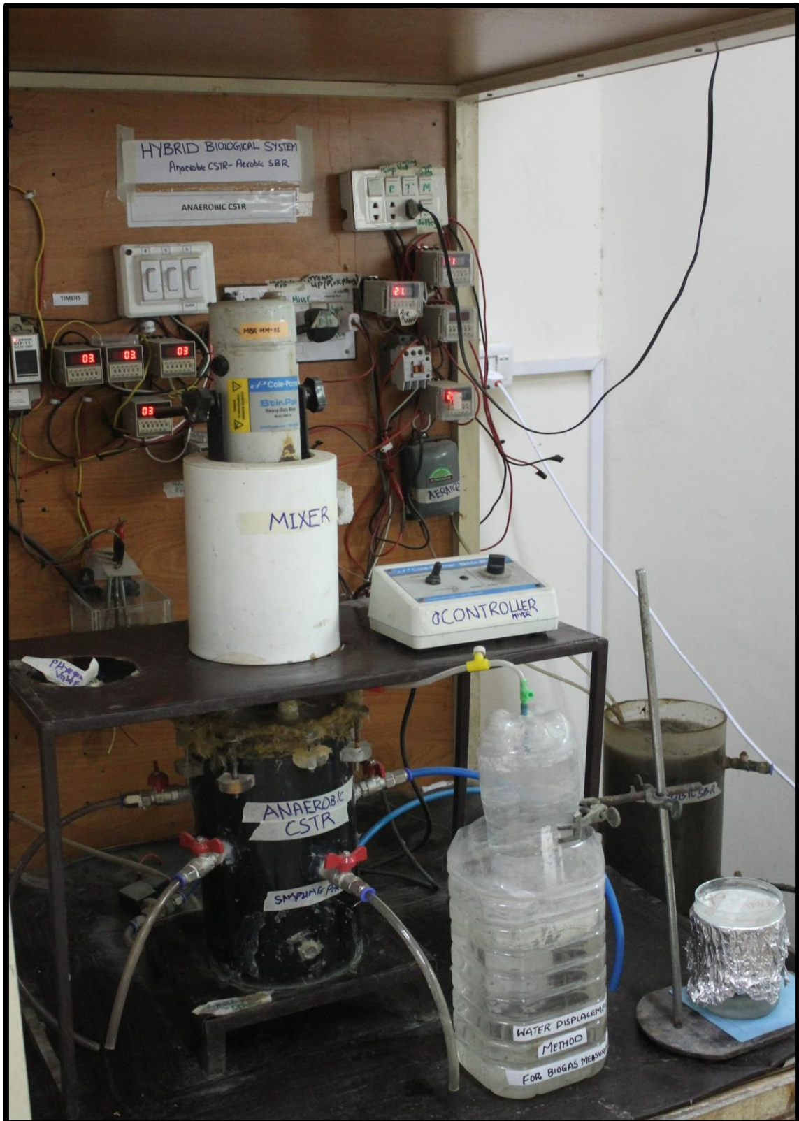
Figure 3.1: Laboratory scale setup of hybrid anaerobic-aerobic biological system.
