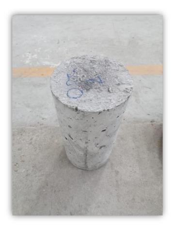
The samples casted are initially submerged in water at room temperature (25°C to 30°C) for 24 hours and weighed, then those wet samples were placed in an oven for 24 hours and weighed, keeping in view the guidelines of section 7 of ASTM C-67. Calculated as:
