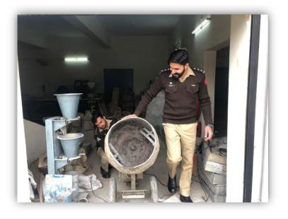
Conclusions can not be made about concrete short of proper testing as per ASTM standards. Compilation of results followed by recommendations can only be done based on tests carried out on samples. For testing we casted a 12" x 6" cylinder, a prism, three 4" x 4" cubes and a 6" x 3" cylinder for each mix using hand mixing and mixer machine at MCE concrete lab. submerged curing was ensured at for all samples for 28 days.
