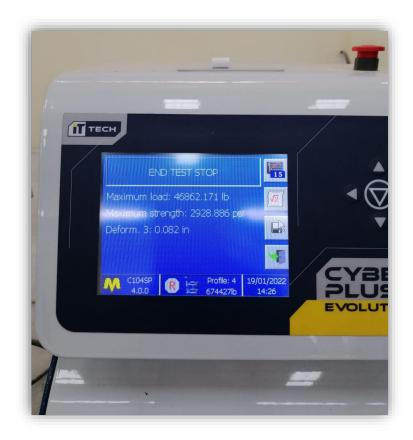
It is a type of mechanical test used to determine the ultimate sum of compressive load that a material can take before fracturing. Typically used samples are cylinders or cubes, the sample is compressed between the plates of compression-testing machine by applying load gradually as per ASTM C39 . 3 similar samples were tested after curing and average strength was noted.
