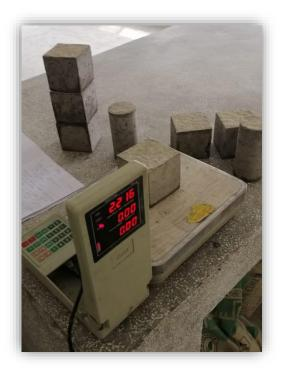
The surface density has been calculated as per ASTM-138. The unit weight of the composite sample was divided by its volume to get the surface density.
