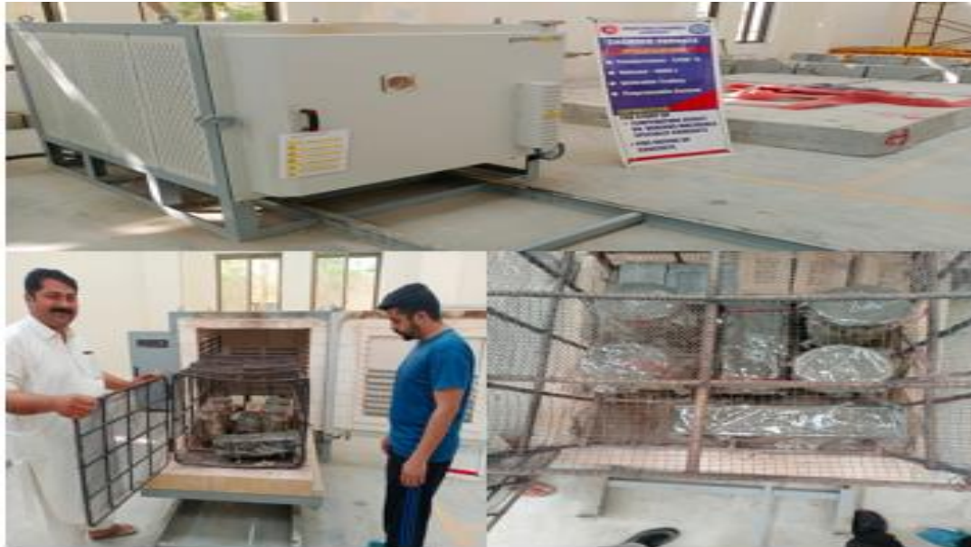
Figure 3.8 Dry Curing of FGPC in Oven
