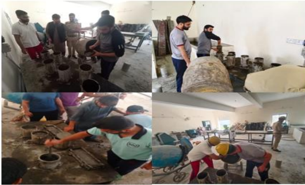
Figure 3.7 Casting of Concrete
