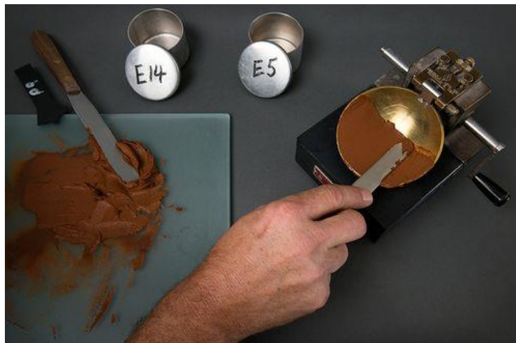
Figure 3-3 Atterberg's limit of soil
