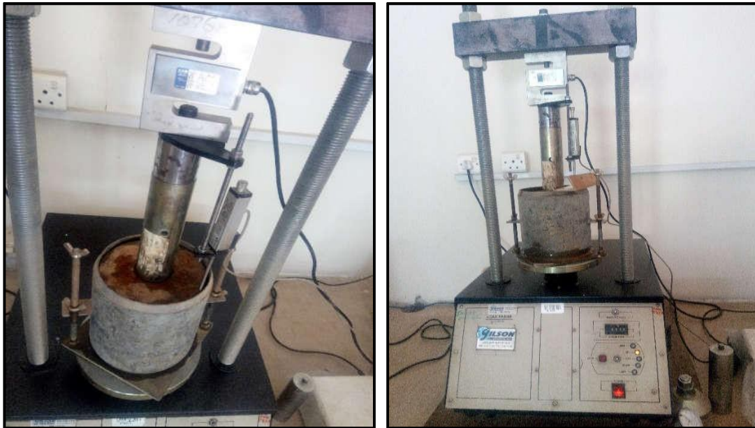
Figure 3-6 (a,b) CBR Testing
