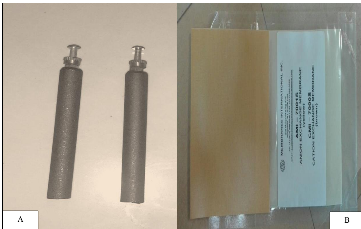
Figure 3.2: graphite rods (A) and cation exchange membrane (B), used in the study
