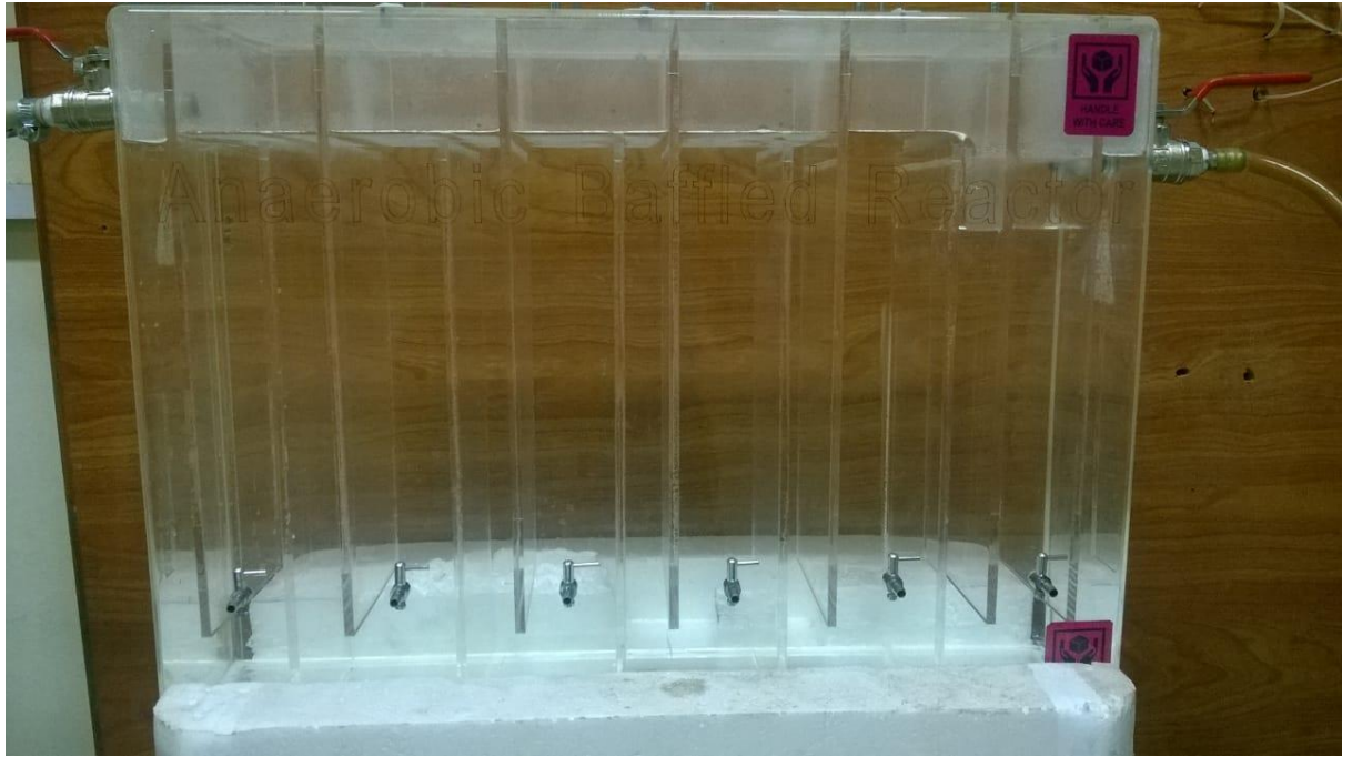
Figure 3-2: Fabricated ABR for Lab scale study
