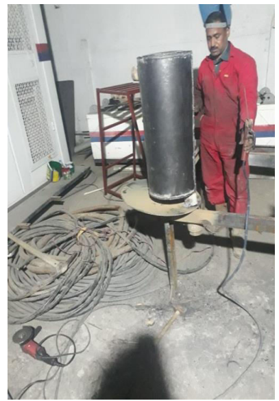
Figure 21 Reactor Inner Cylinder
