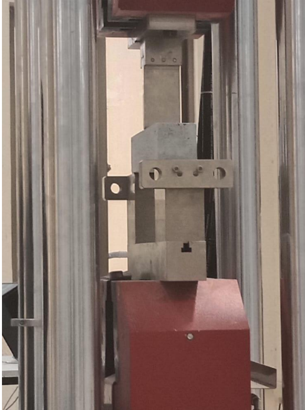
Figure 4- 4 Flexural testing on UTM
