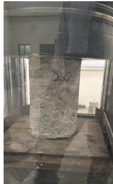
Figure 4- 2 Testing on CTM at 20%
