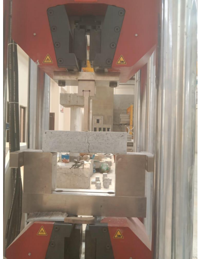
Figure 4- 5 Flexural testing on UTM
