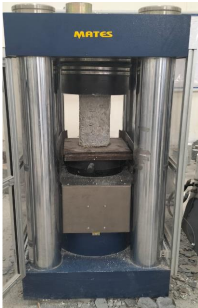
Figure 4- 1 Testing on CTM at 15%
