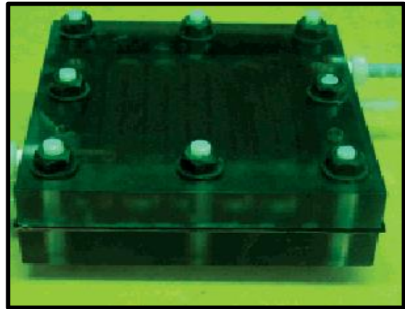
Figure 2.4b Flat plate layout in which a reactor is cut into the blocks to allow fluid to flow through the electrode in a serpentine pattern
