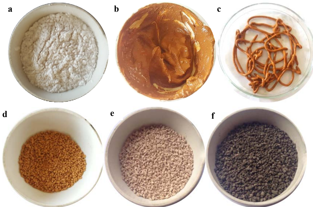
Figure 3.2: Catalyst preparation (a) Parent HZSM-5 (b) Paste formation (c) Extrusion (d) Fe-ZSM-5 (e) Zn-ZSM-5 (f) Co-ZSM-5
