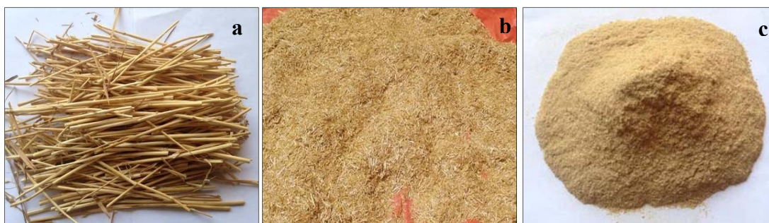
Figure 3.1: Feedstock preparation (a) Raw form (b) Shredded form (c) Grinded form
