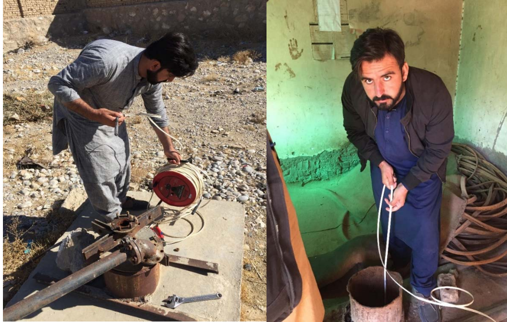
Figure 3.5. Water table measurement by manual deep meter
