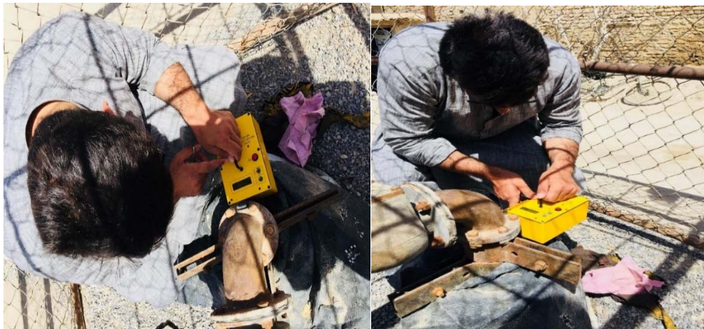
Figure 3.6. Water table measurement by sonic deep meter
