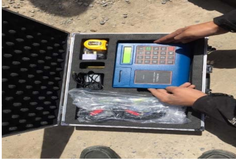
Figure 3.4. Measuring the Discharge of selected tube wells using ultrasonic flow meter
