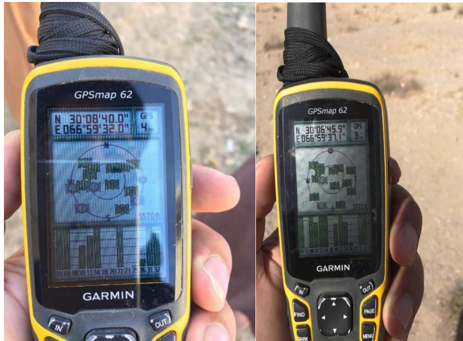
Figure 3.3. Finding coordinates of selected tube wells in the field using GPSMap
