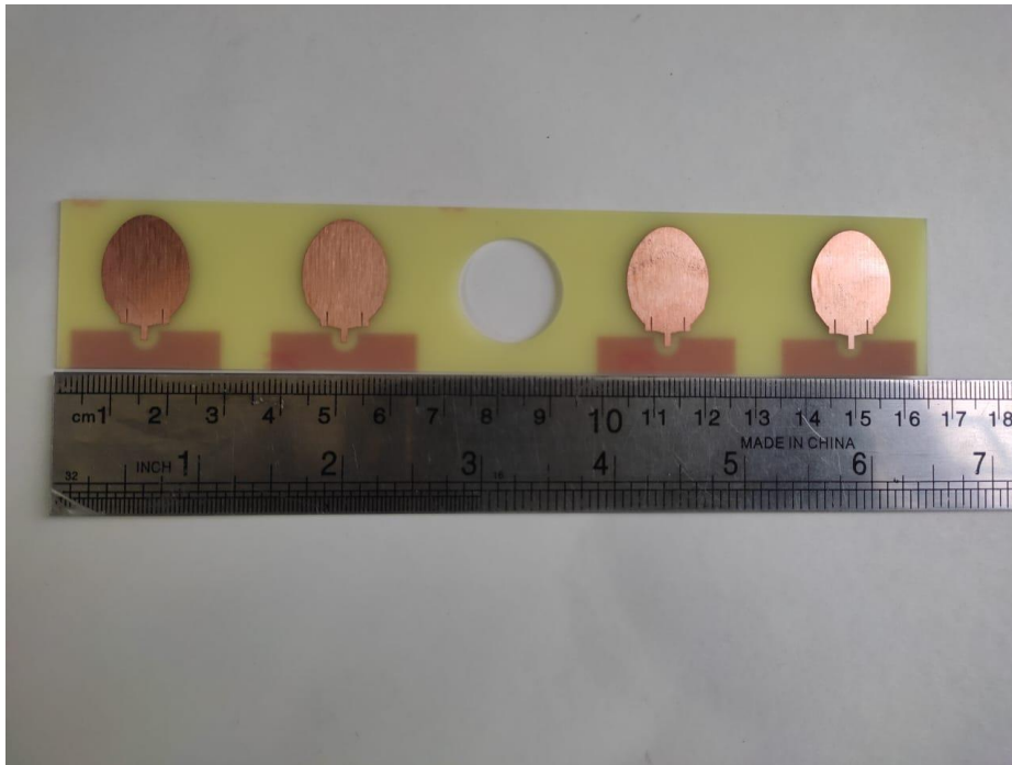
Figure 3.19 Array of microstrip patch antenna (fabricated)
