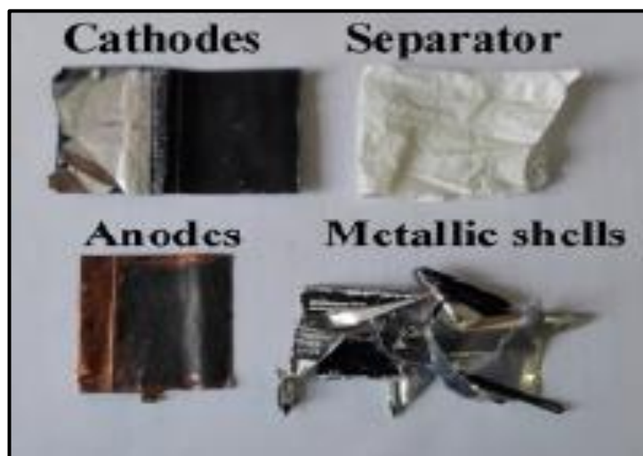
Figure 2.1. Components of lithium ion batteries
