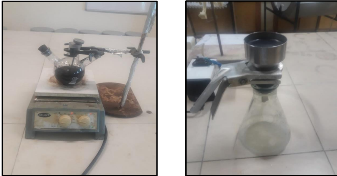
Figure 3.6. Leaching Apparatus (leaching setup and filtration assembly)
