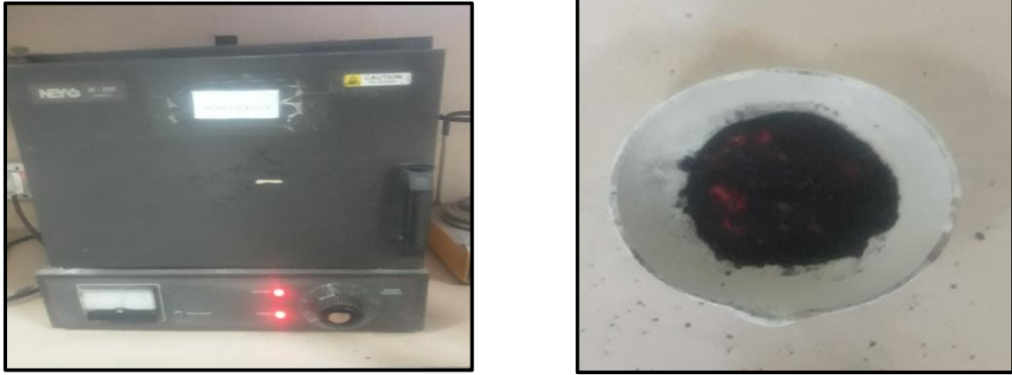
Figure 3.5. Calcination using muffle furnace apparatus
