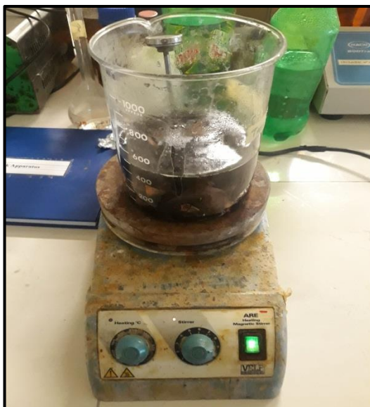
Figure 3.4. Dissolution process to separate aluminum from cathode
