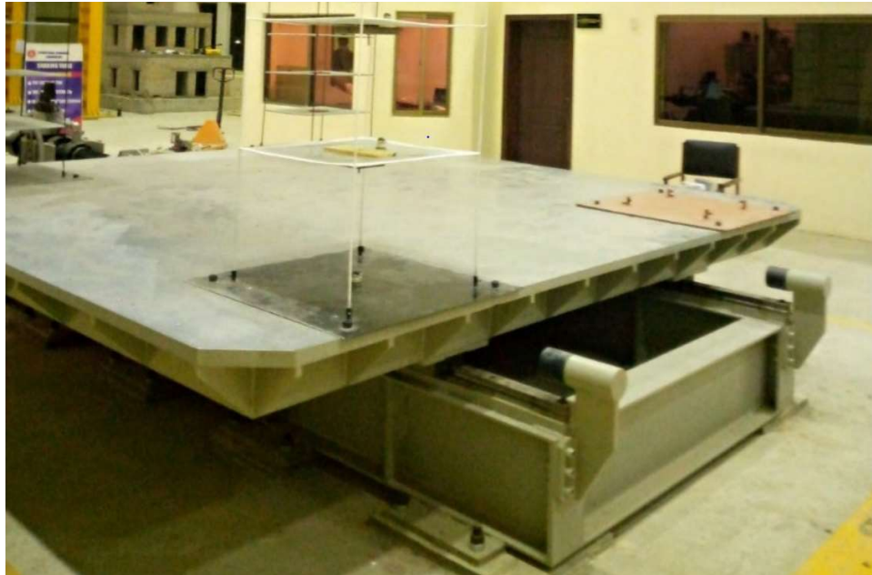
Figure 14 BESMAK Shake Table Platform
