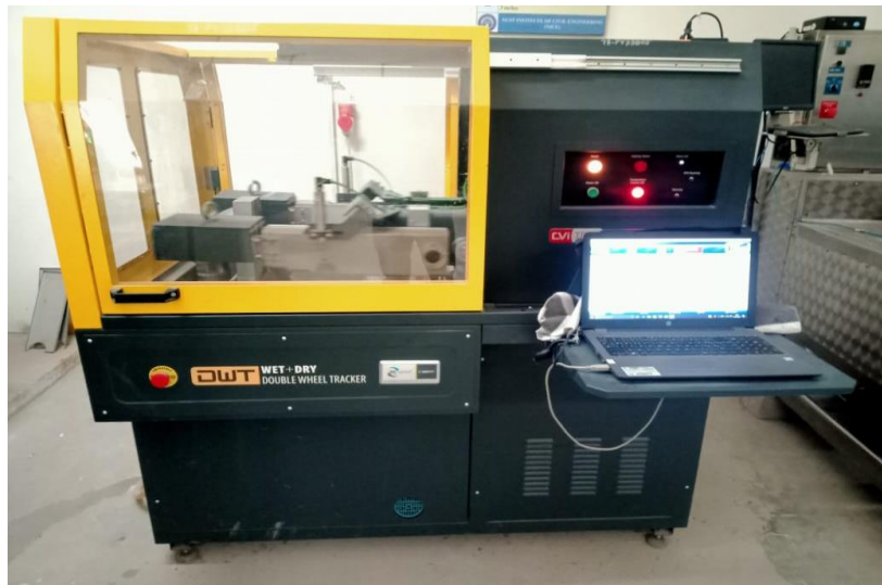
Figure 3.6: HWTT apparatus for determining rut depth of asphalt mixtures
