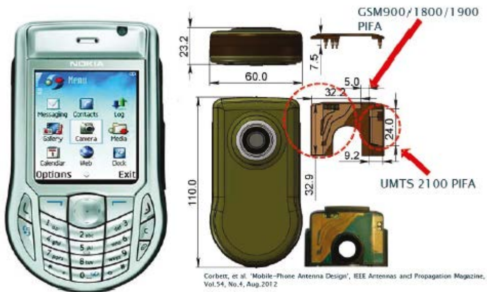
Fig 2. 5 Nokia 6630 with its internal Antennas
