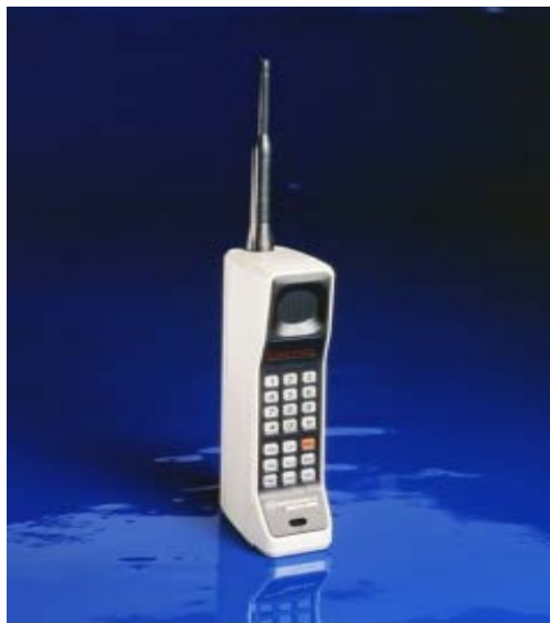
Fig 2. 1 Sleeve dipole antenna used by Motorola DynaTAC8000X
