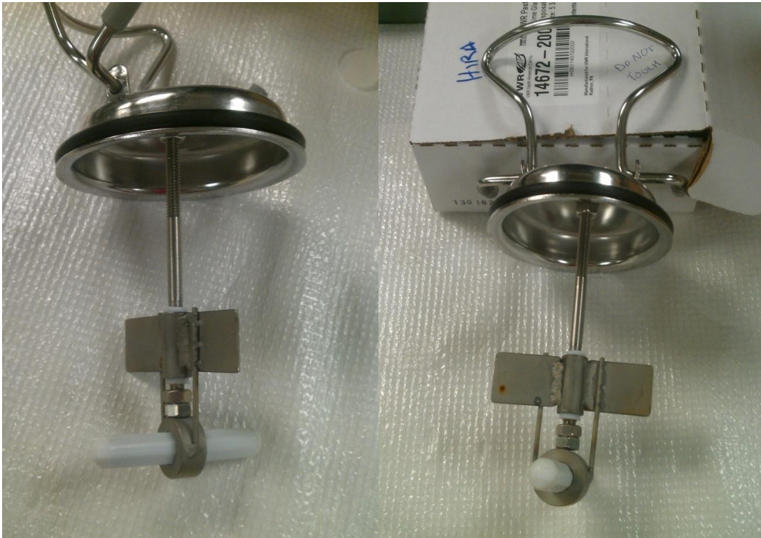
Figure 3-9: Modified lid of pressurized feed reservoir having metallic paddle and magnetic stirrer
