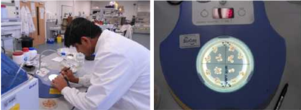
Figure 3-5: Bacterial colony counting on a digital colony counter
