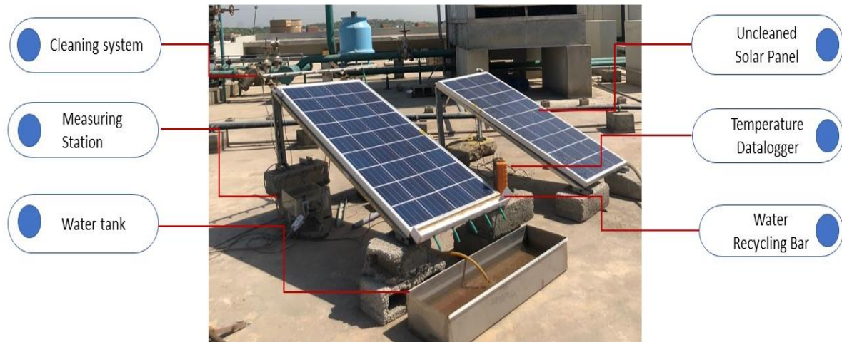
Figure 3-6 Unclean and Clean PV module attached with automatic cleaning system
