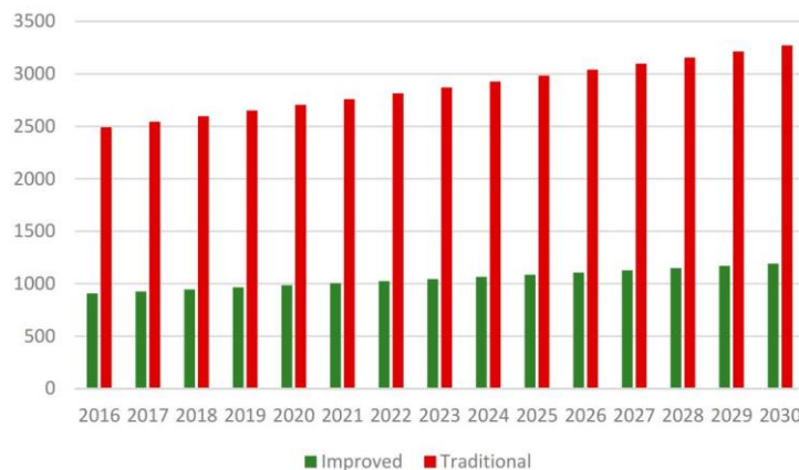
Figure 2- 8 Fuel wood demand in Honduras in BTOE in case of Traditional and Improved Stoves
