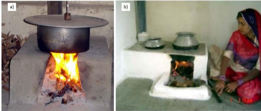
Figure 2- 11 a) Single Pot ICS b) Double Pot ICS
