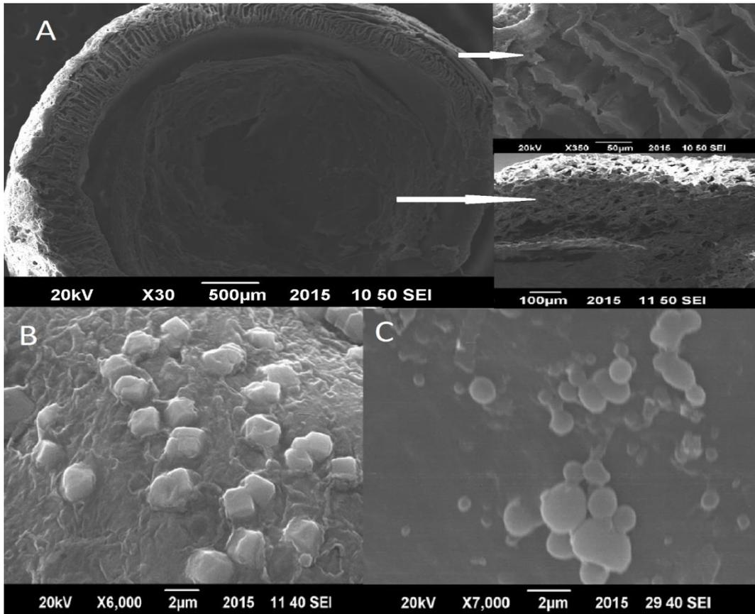
Figure 4.9. SEM images of QQ-bacteria entrapped polymeric bead (A) Cross-sectioning image of whole bead and polysulfone membrane matrix in the bead, (B & C) Inner surface of the polymeric bead
