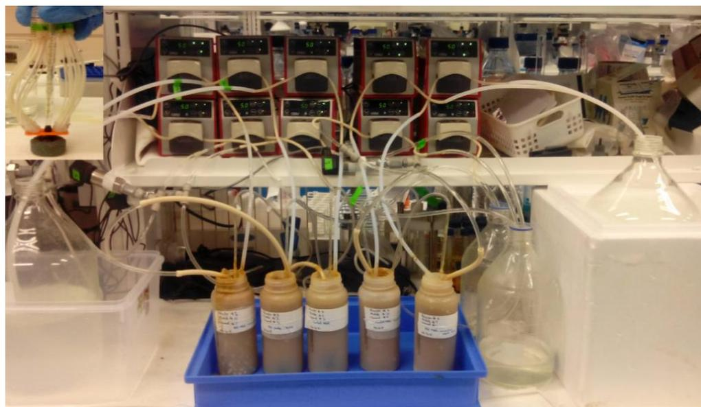
Figure 3.5. Batch scale MBRs set up for Phase 3
