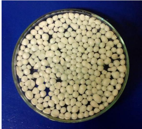
Figure 3.3. Alginate beads coated with polysulfone
