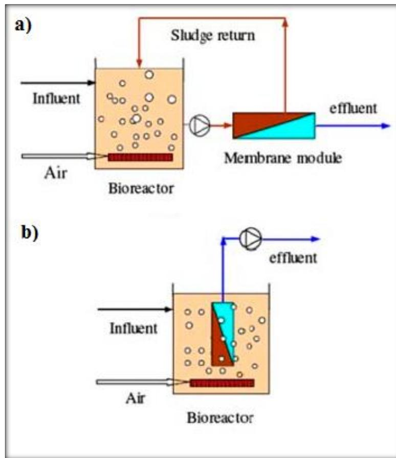
Figure 2.2. General configuration of (a) Side stream MBR, (b) Submerged MBR
