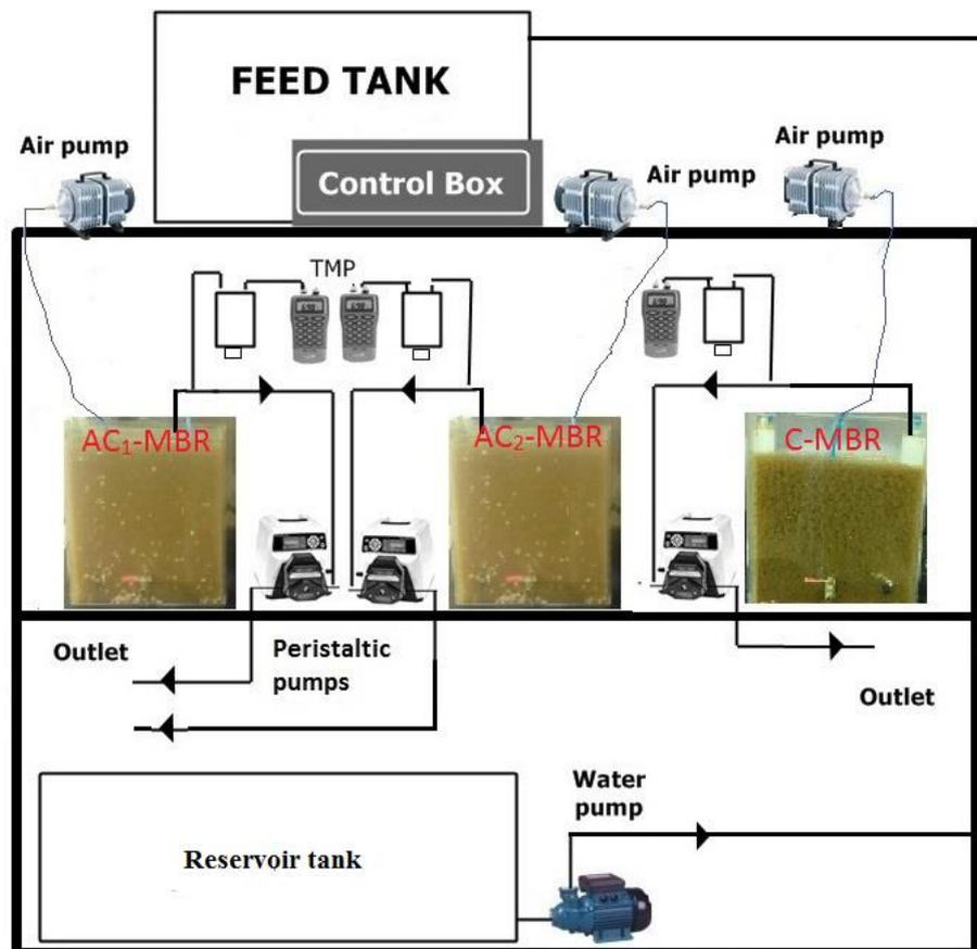
Figure 3.4. Schematic of lab scale MBRs setup used for Phase 2
