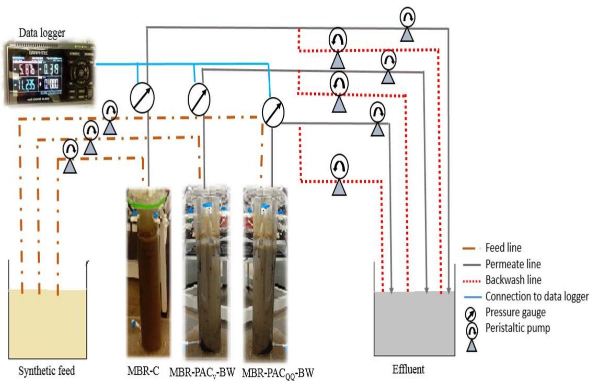
Figure 3.7. Schematic of lab-scale MBRs setup for Phase 4
