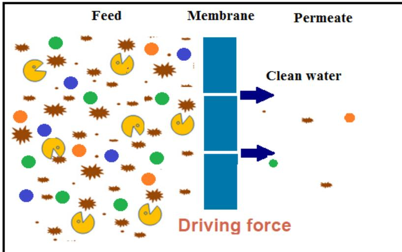
Figure 2.1. Process diagram of membrane bioreactor (MBR)
