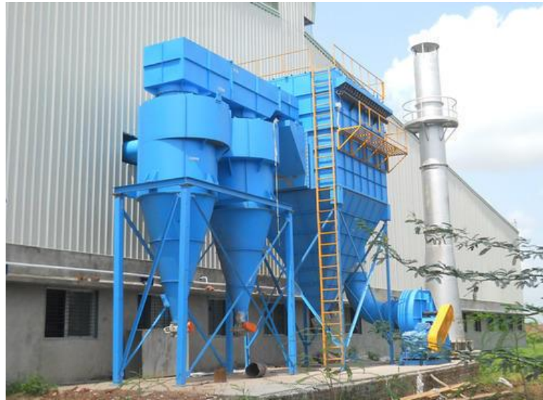
Figure 1.5: Swirl flow in pollution control devices [11]
