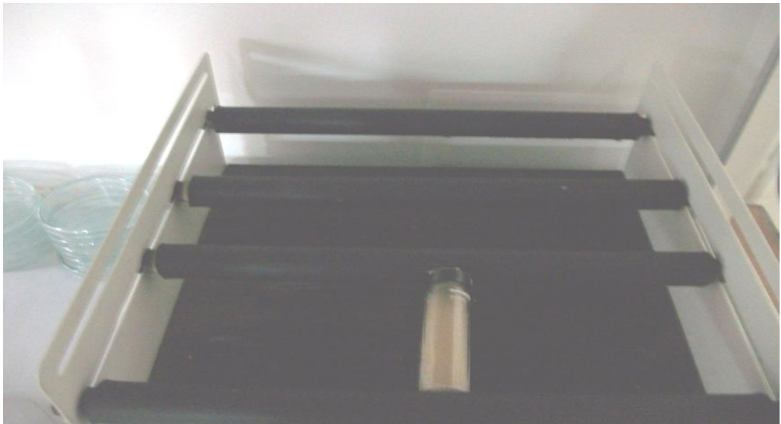
Figure 3. 2: UV-cell containing bacteria and NPs (exposed to Fluorescent light)
