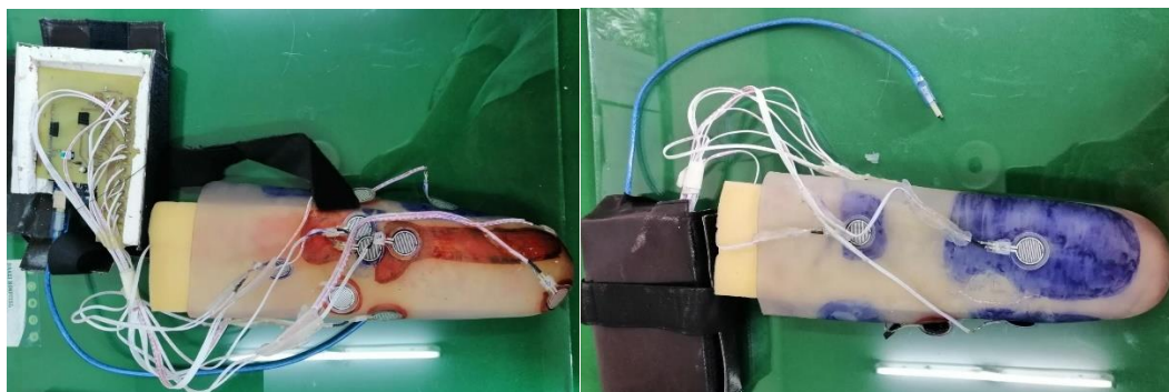
Figure 18: Stump Liner Embedded with FSR Sensors
