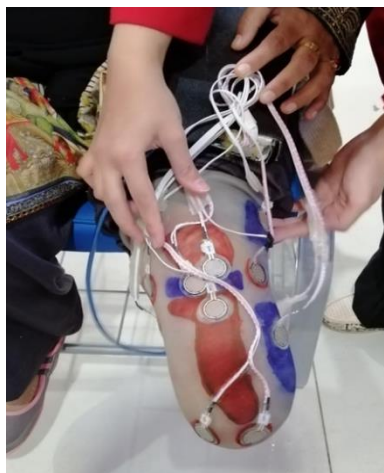
Figure 9: Concept of the Wearable Pressure Mapping System
