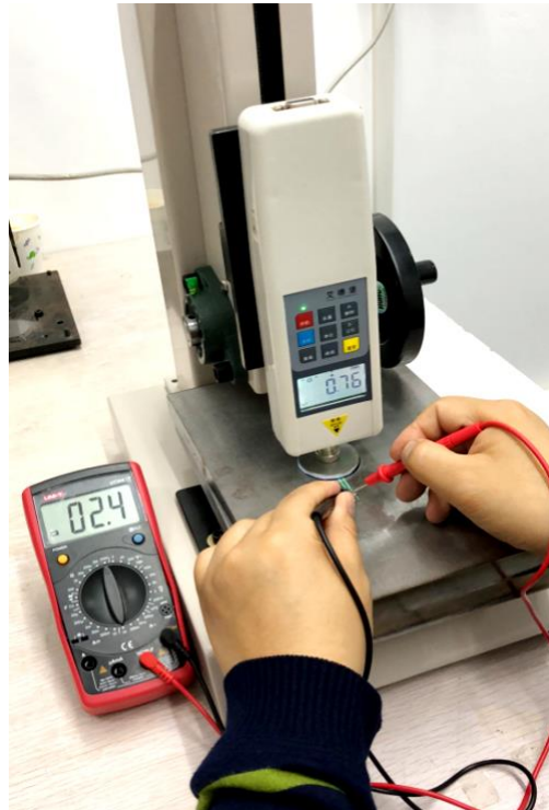
Figure 15: Sensor Calibration Method
