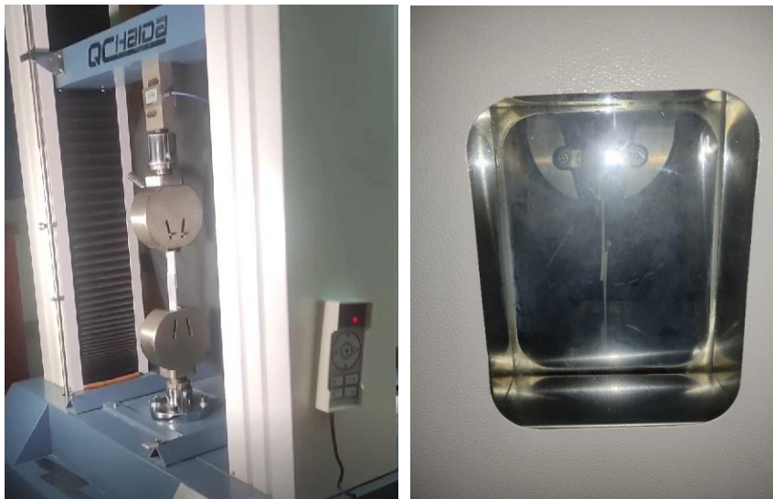
Fig. 3.32 UTM testing of SLJs ant room and higher temperatures
