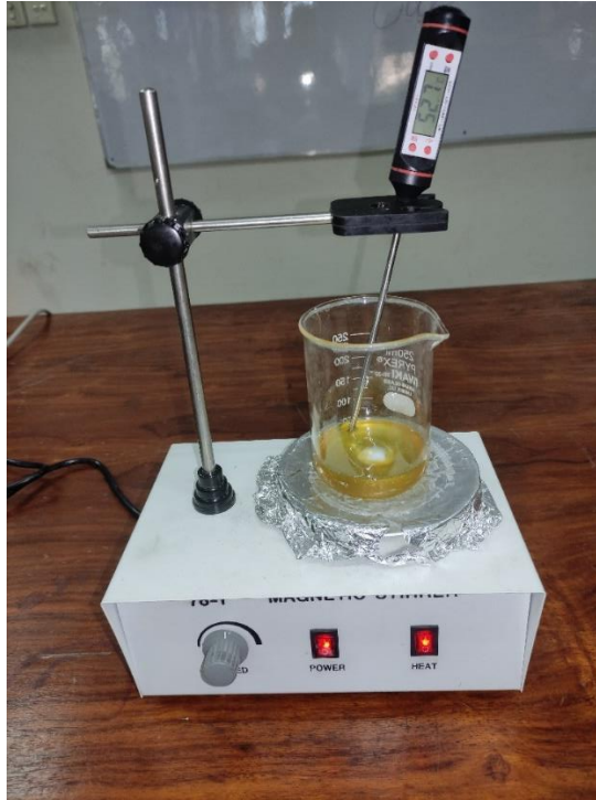
Fig. 3.13 High temperature mixing of epoxy and cork powder
