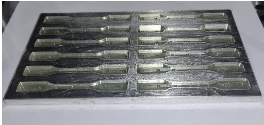
Fig. 3.11 Adhesive poured inside the mould
