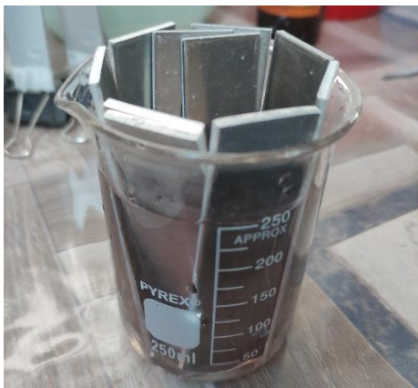
Fig. 3.24 Acetone solution cleaning
