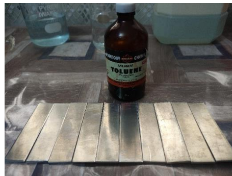
Fig. 3.27 Cleaning with Toulene solution
