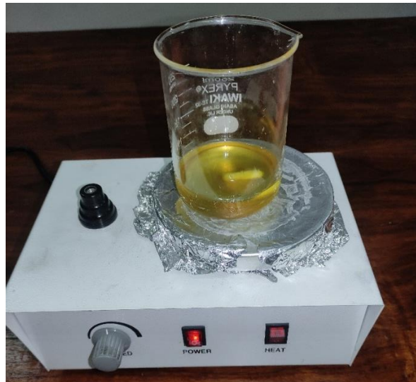
Fig. 3.14 Mixing of hardener
