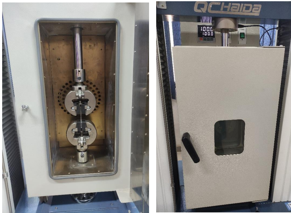
Fig. 3.22 UTM testing of adhesives at higher temperatures
