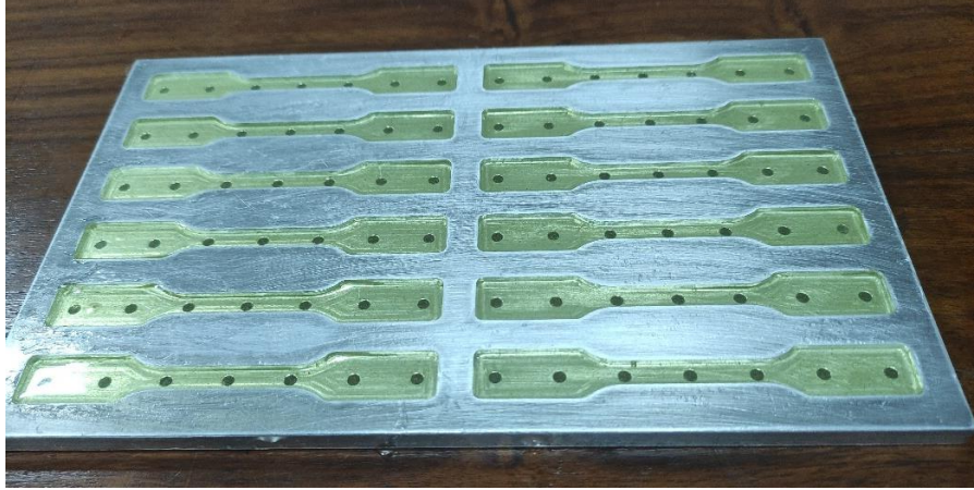
Fig. 3.15 Cork powder samples poured inside the mould
