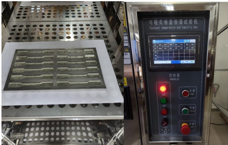
Fig. 3.16 Mould is placed inside the curing oven
