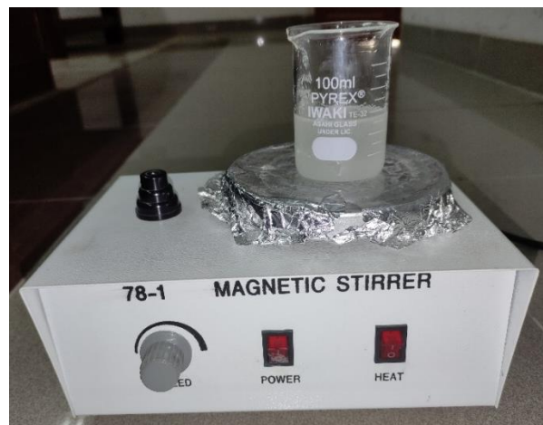
Fig. 3.10 Epoxy stirring on magnetic stirrer
