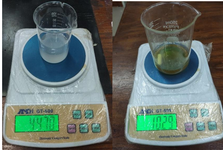
Fig. 3.9 Weight measurement for epoxy and hardener
