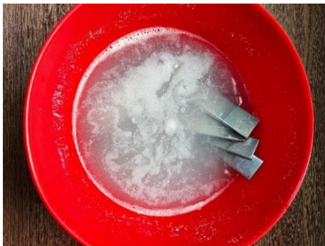
Fig. 3.26 Degreasing with detergent
