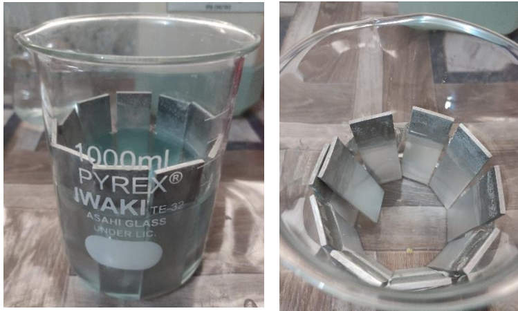
Fig. 3.28 Post treatment rinsing with HNO 3 and water
