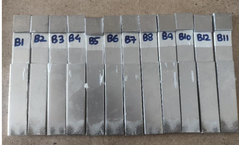
Fig. 3.31 SLJs prepared after curing process
