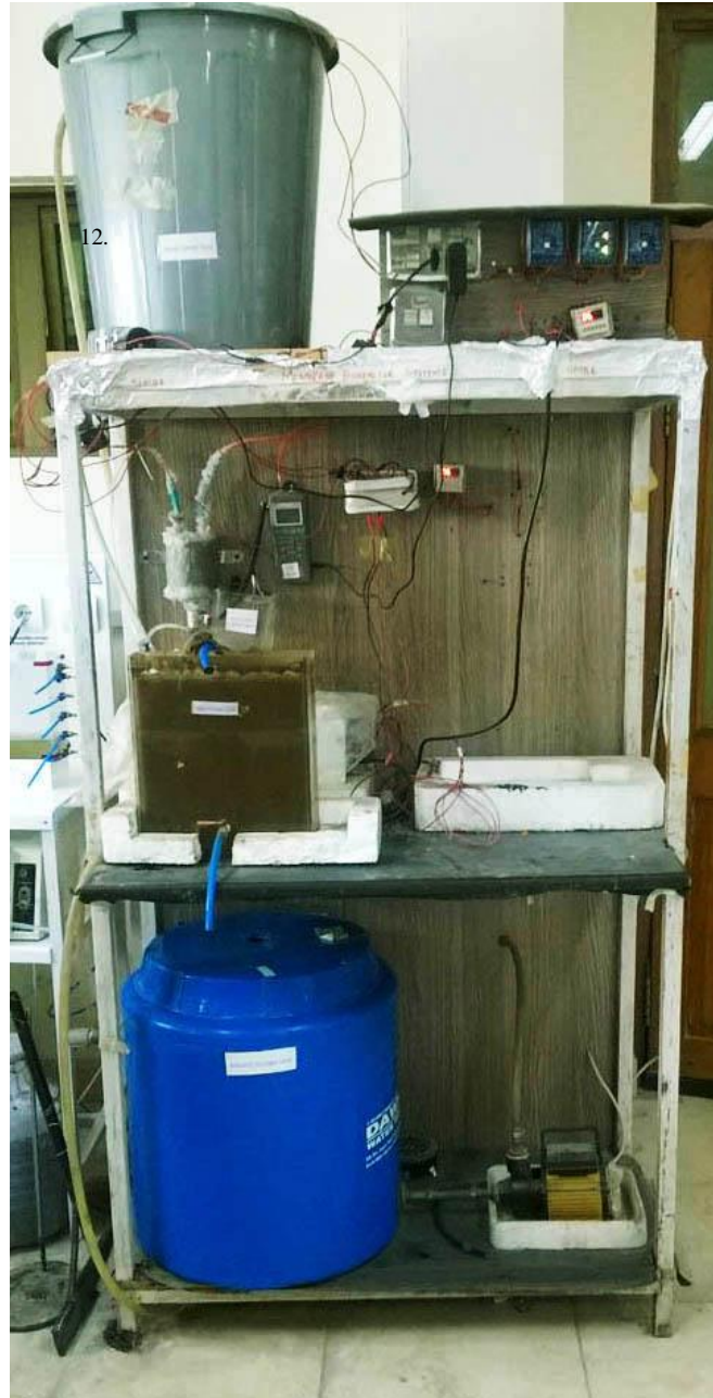
Figure 3.2: Membrane Bioreactor Setup
