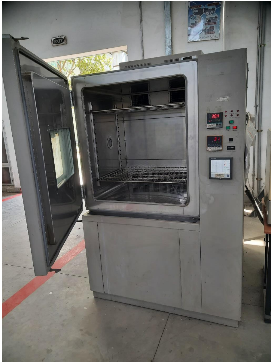
Figure 10: Low Temperature Chamber
