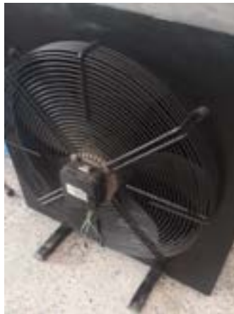
Figure 2.7: Heat exchanger attached with system for maintaining hydraulic oil at required temperature
