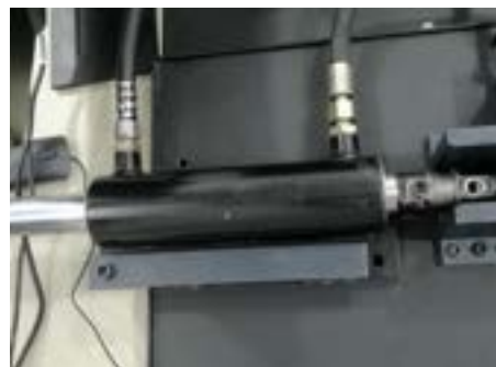
Figure 2.2: External actuators for load on test piece
