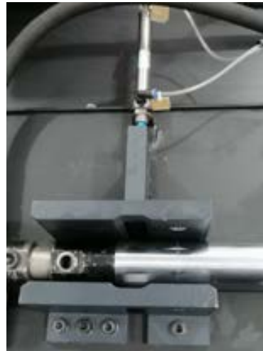
Figure 3.10: Final product of block stopper
