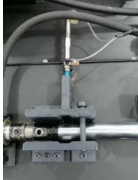
Figure 3.17: Manufactured gate slider
