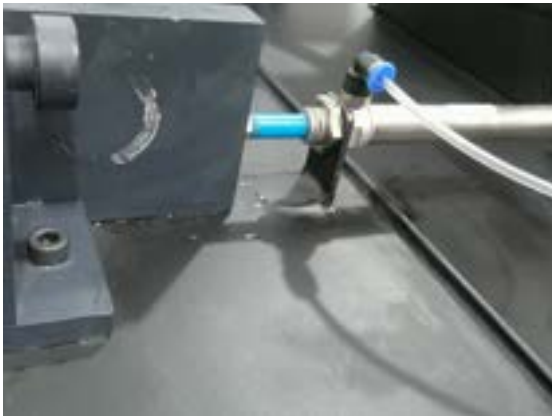
Figure 3.18: Gate operating with pneumatic actuator
