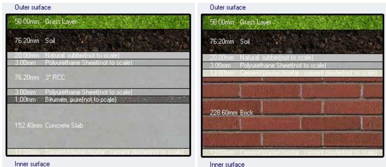
Figure 3.11: (a) Layers of green roof (b) Layers of green wall
