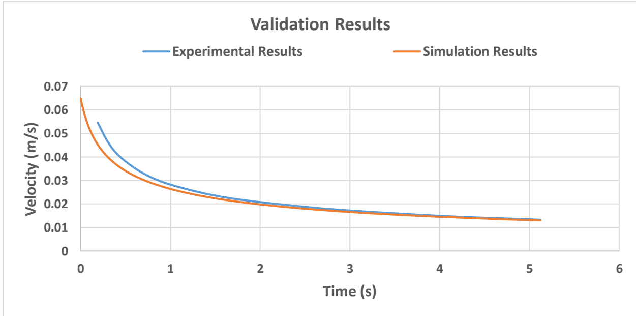
Figure 4.18: Comparison of Experimental and Simulation results for gap height of 390 \mu\text{m}
