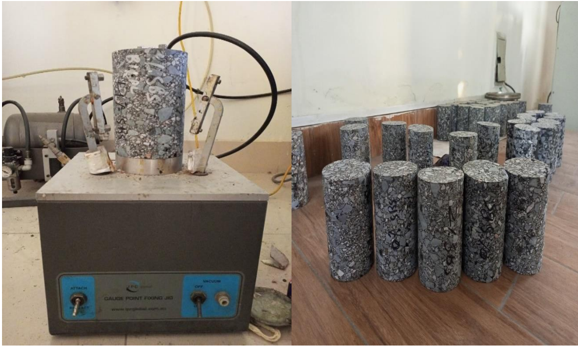
Figure 3.14: Samples Stacked in Lab for Testing and Gauge Point Fixing Jig
