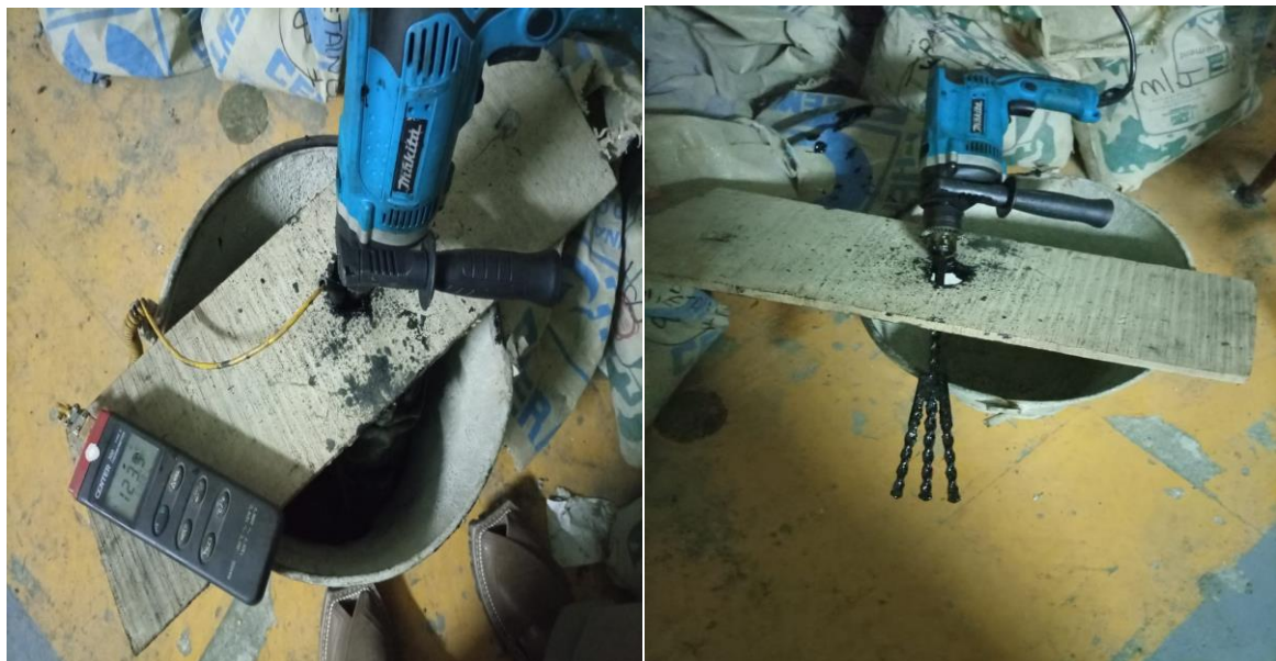
Figure 3.12: Mixing of SBS into Binder with High Shear Mixture
