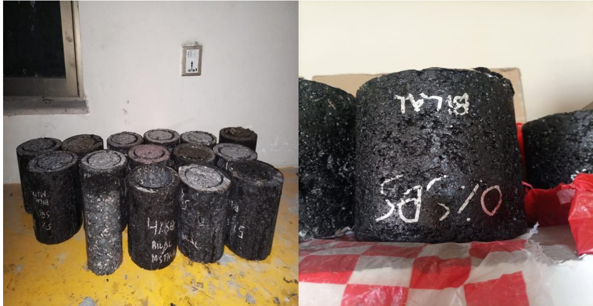
Figure 3.13: Sample Produced from SGC and Cored Samples
