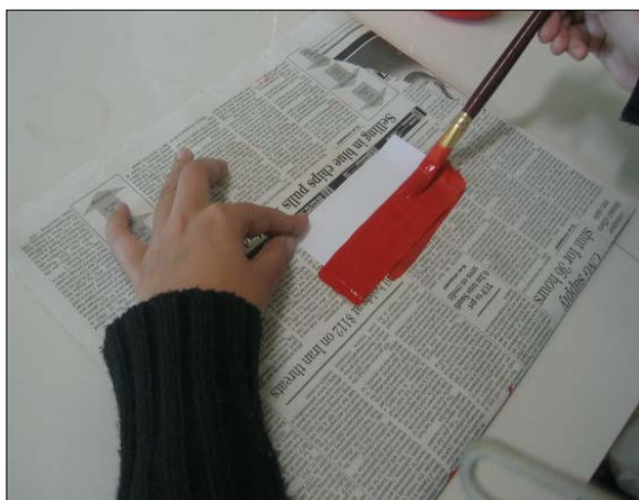
Figure 4 - Application of Thermochromic Paste on the Strip
