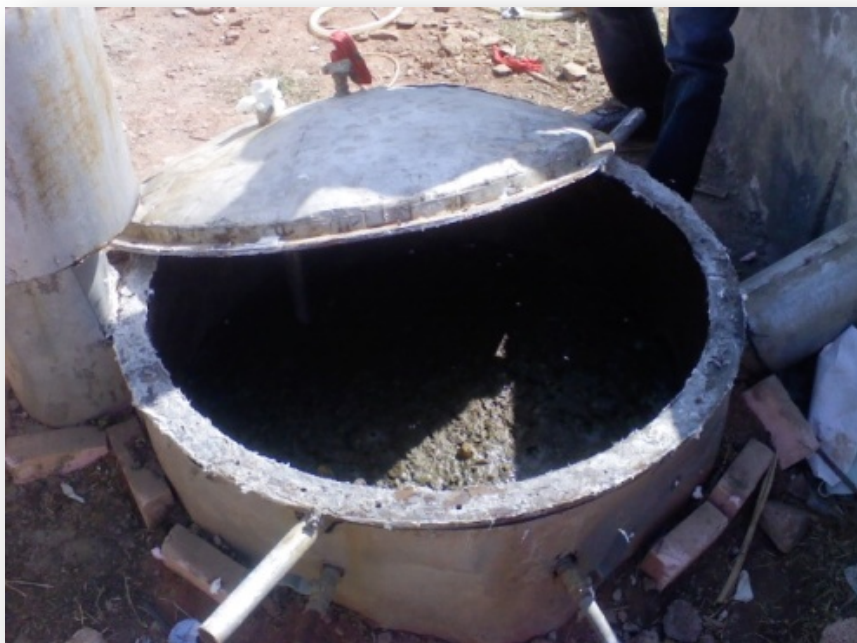
Figure 15 - Headspace Left in Tank for Gas Collection
