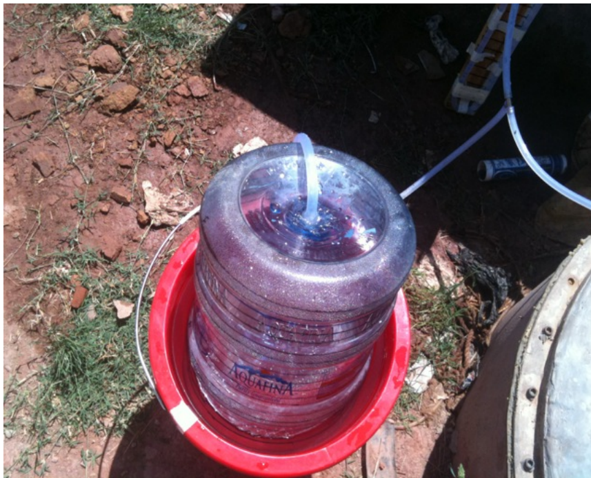
Figure 16 - Displacement Method to Measure Volume of Gas
