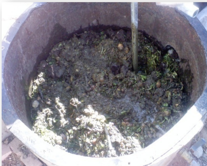
Figure 14 - Manual Mixing of Feed Material to Remove the Scum Layer
