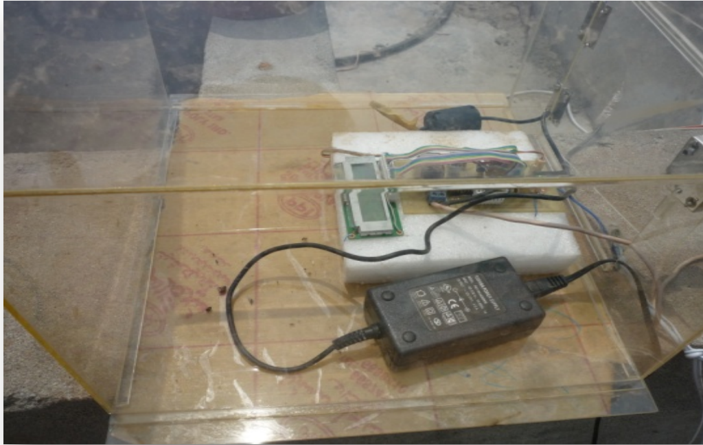
Figure 8 - Temperature Controlling System with LCD Screen that shows temperature inside digester
