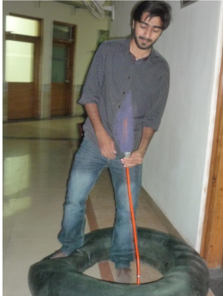
Figure 24- Ignited biogas to observe the Flame
