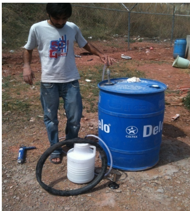
Figure 18 - Filtration of Biogas by Using Lime Water
