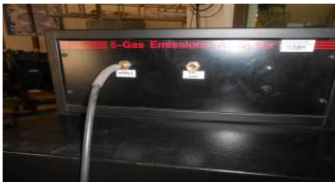
Figure 3.12: Taylor's Five Gas Emission Analyzer (GEA) at SMME
