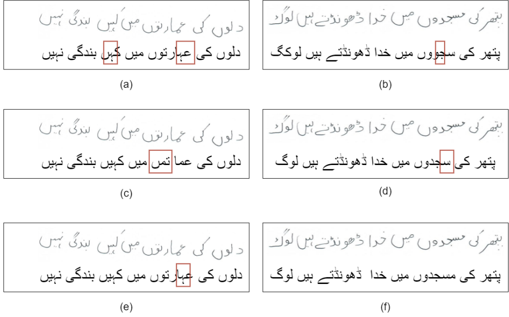
Figure 5.1: Results from the Smoke study are shown in the figure. Results from the Google Vision API are shown in Figs. (a) and (b), with CER values of 7.8% and 5.7 percent, respectively. Results from Zia et al [51]’s model with CER of 5.2 percent and 5.7 percent, respectively, are shown in Figs. (c) and (d). Results from the suggested model, which has a CER of 2.6% and 0%, are shown in Figs. (e) and (f)
