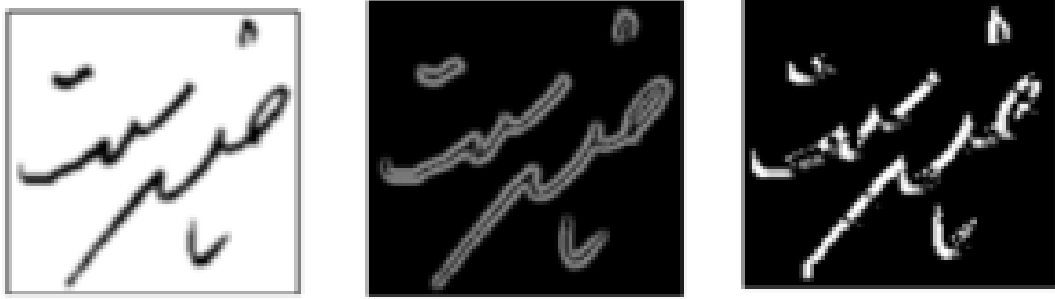
(a) 128 x 128 Grayscale Image (b) Image's Gradient Strength (c) Gradient Direction
