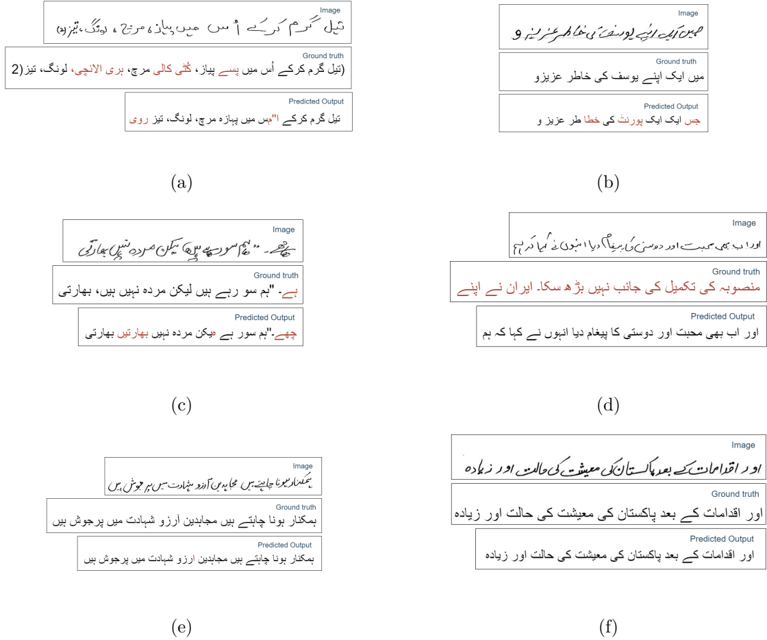
Figure 5.2: The image displays instances of some of the input together with its ground-truth and predicted text presented below. Examples of label noise in the dataset are shown in (a). Given a picture, the given ground truth has extra, unneeded words or characters. present in the supplied image, raising this example's CER. The model accurately foretells the characters in the input image. (b) includes an an illustration of a distorted input image The model cannot foresee the actual label since the input images only contain a few difficult-to-read letters or literals because of the author's writing style. The input image for (c) has a calligraphic writing style that is intricate and challenging for the model to correctly predict. There is a sample of label noise in the dataset in (d). The provided ground truth for a given image is unreliable, but the predicted result is accurate given the input image. This demonstrates that the model is effective enough to yield reliable outcomes. The mismatched ground truth is the cause of the high CER. The situations where the model accurately detected the handwritten text and produced an extremely low CER are contained in the table (e), (f)
